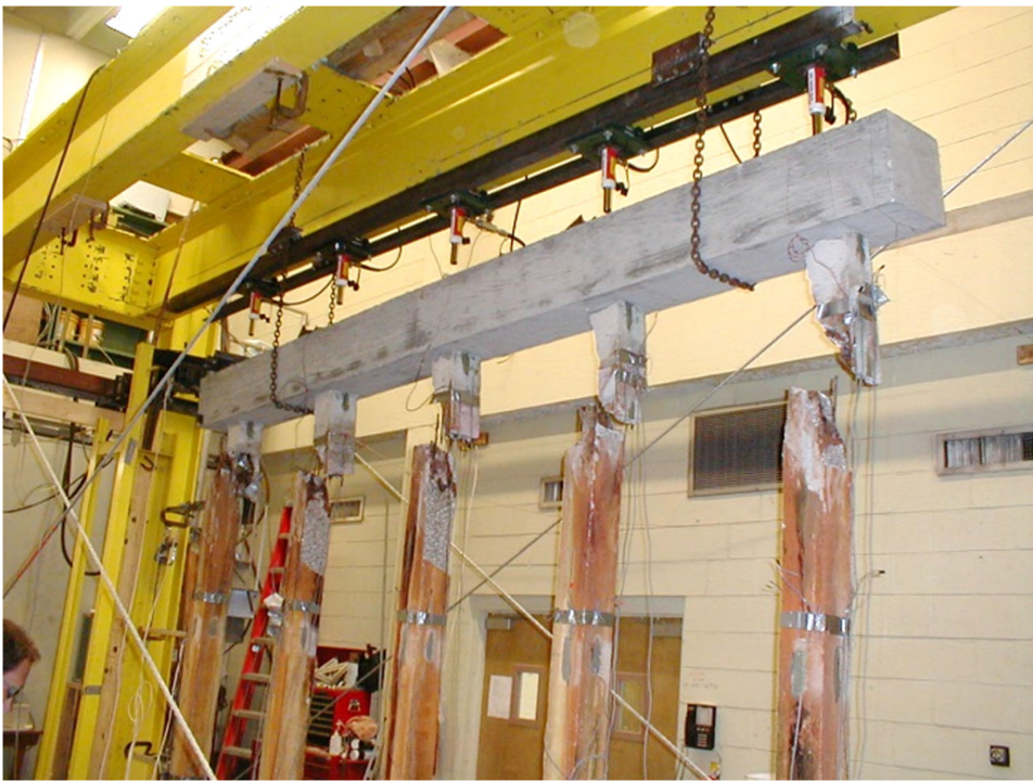
Figure 17. The 50% bridge bent after catastrophic failure (cap caught by safety chains).
