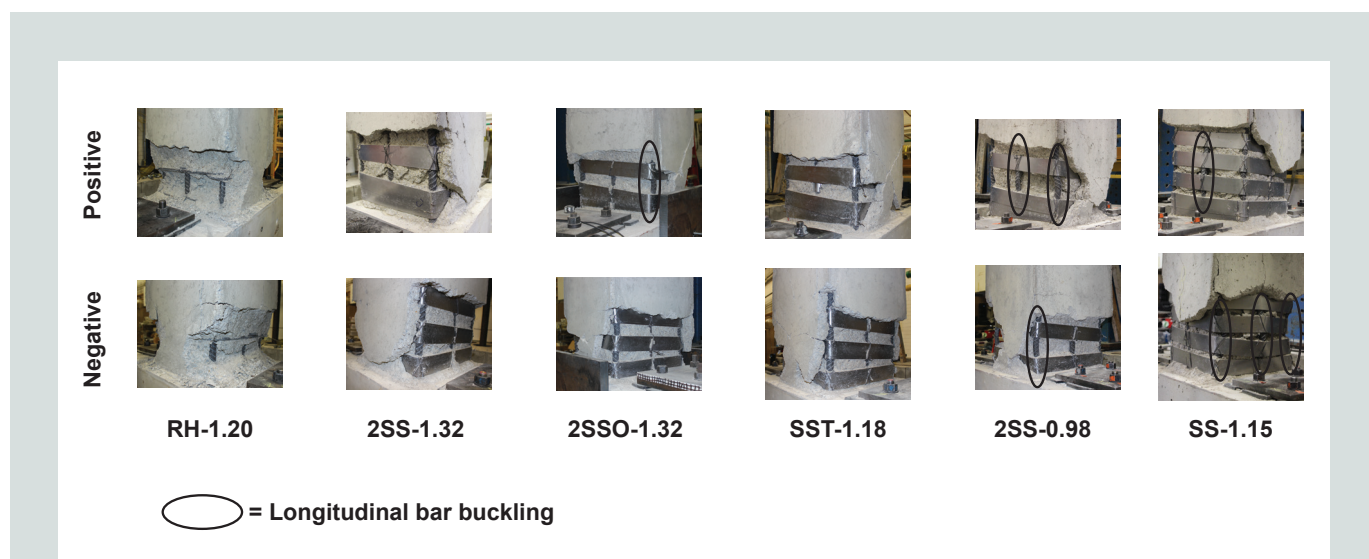
Figure 12. Photographs of excavated specimens after testing. Positive and negative labels indicate the compression face under that loading direction. Note: RH = reinforcing bar hoops; SS = one strip spiral; SST = one strip spiral with crosstie; 2SS = two strip spirals; 2SSO = two strip spirals that are out of phase.
