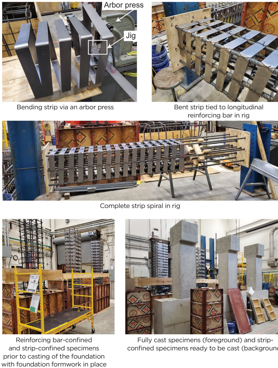
Figure 5. Specimen construction.
