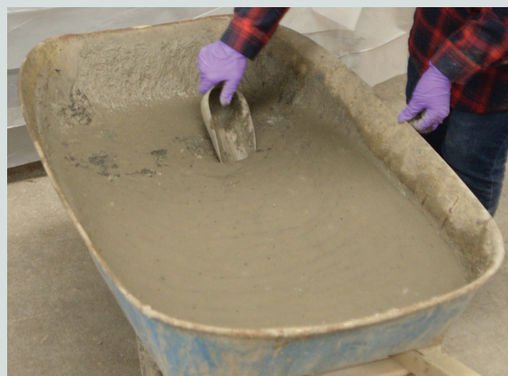
Figure 1. Formation of elephant skin on freshly batched ultra-high-performance concrete. Note the surface texture in response to scooping.
