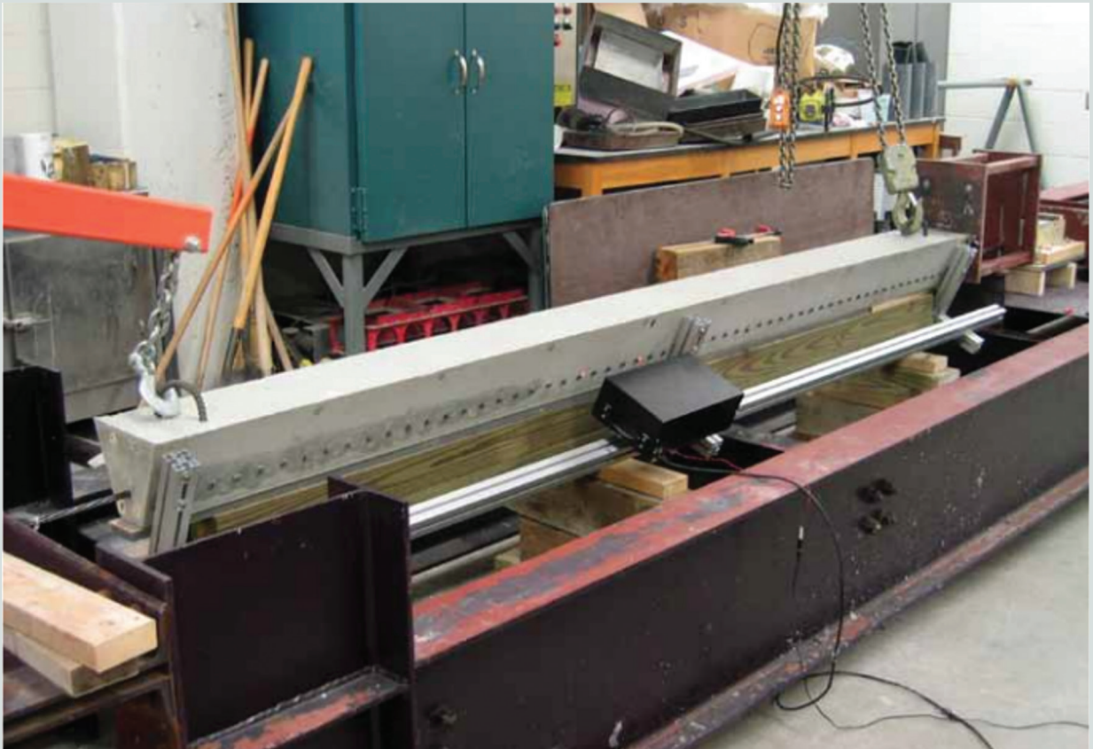
Laser speckle device used to measure concrete strains.
