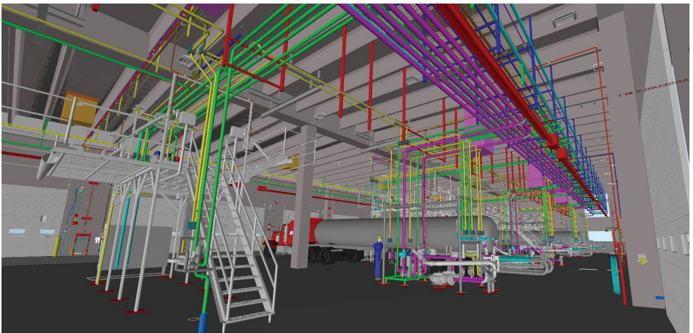
An Autodesk Navisworks in-progress model shows building and piping in the receiving area. Courtesy of Shambaugh & Son LP.
