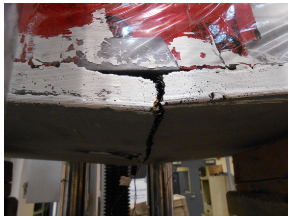
Major crack of the bottom wythe in W2 and W3
