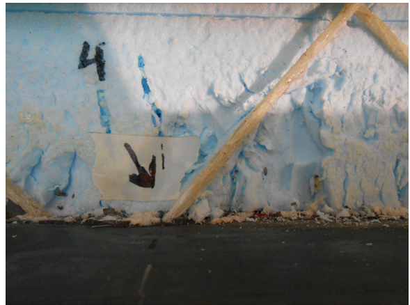
Failure of the diagonal GFRP connectors in W8, some in tension and some in compression
