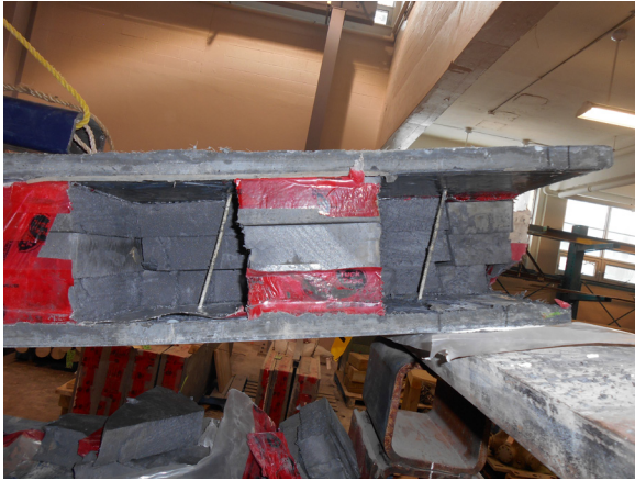
Fracture of GFRP ties near the concrete face in W1 to W7
