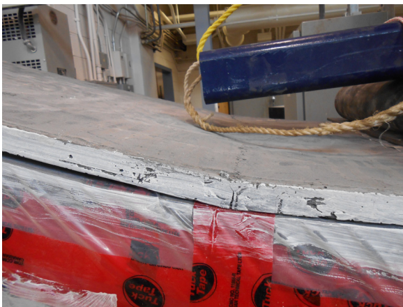
Major separation of the top wythe of W1 and W8
