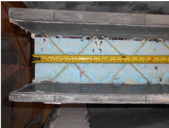
Failure of the diagonal GFRP connectors in W8, some in tension and some in compression
