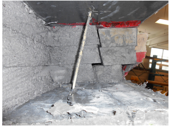
Fracture of GFRP ties near the concrete face in W1 to W7
