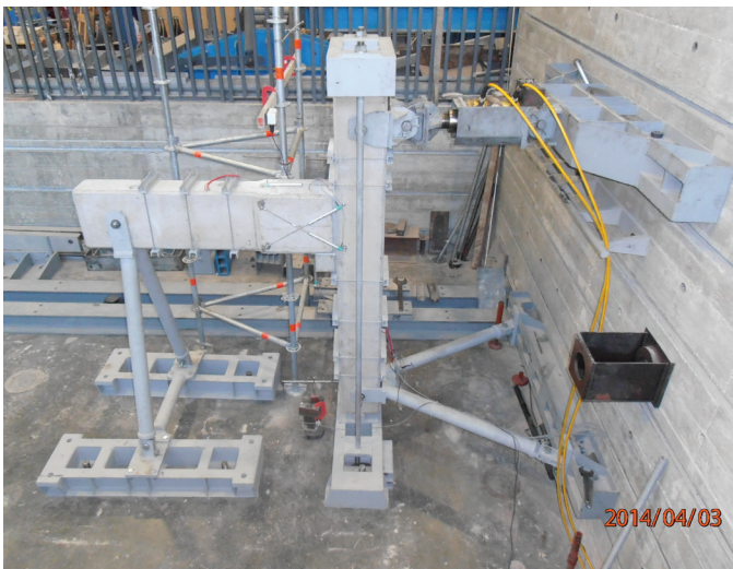
Figure 7. Reduced-scale experimental setup of the precast concrete solution.
