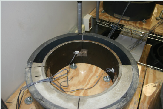
Figure 4. Ring setup for the placement of the second material and a final restrained bond ring specimen.
