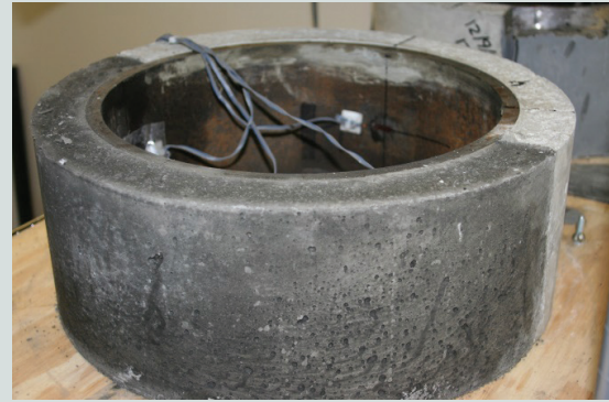
Figure 4. Ring setup for the placement of the second material and a final restrained bond ring specimen.
