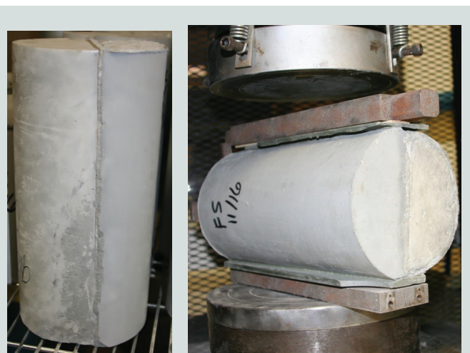
Figure 3. Typical 6 × 12 in. (150 × 300 mm) split cylinder bond specimen and testing setup.
