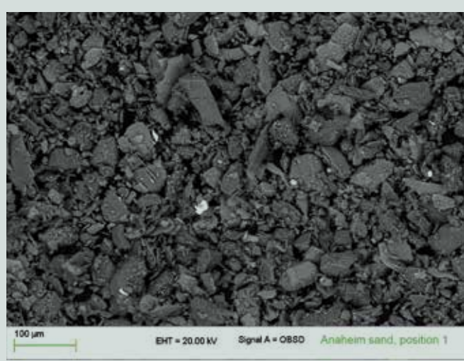
Figure 4. Scanning electron microscope standard backscatter image of Anaheim sand on < no. 325 (0.0450 mm) sieve. Note: EHT = electron high tension; QBSD = quadrant back scattered detector. 1 \mu\text{m} = 3.937 \times 10^{-5} in.
