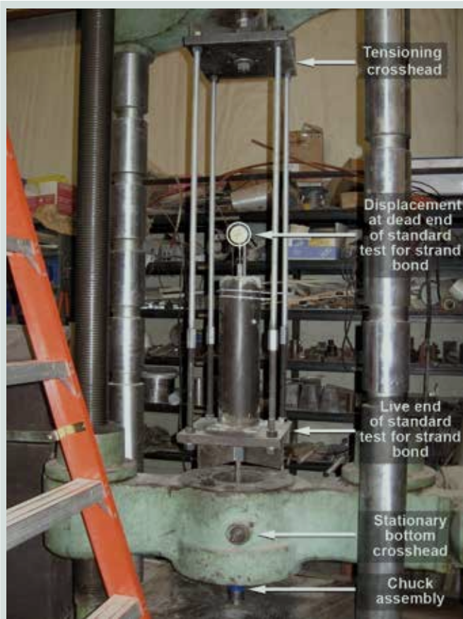
Figure 1. Testing frame in place on testing machine.
