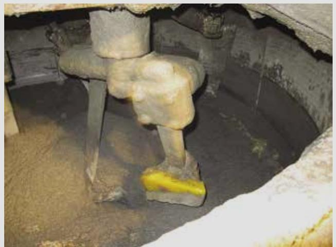
Final mixing stage as fibers are distributed into the concrete
