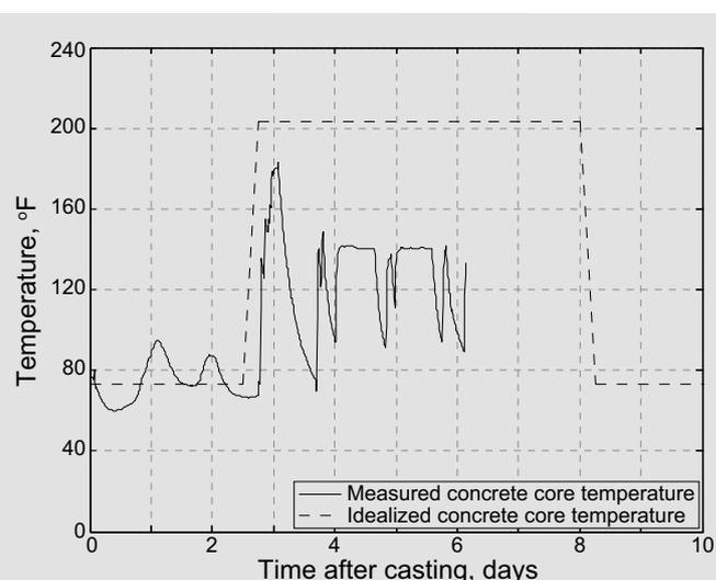
**Figure 4.** Core temperature of a 6.0 × 6.0 × 40 in. ultra-high-performance concrete beam during the curing of trial batch 1. Note: 1 in. = 25.4 mm; °C = (°F - 32)/1.8.
