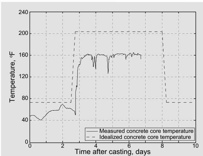
**Figure 5.** Core temperature of a 6.0 × 6.0 × 40 in. ultra-high-performance concrete beam during the curing of trial batch 2. Note: 1 in. = 25.4 mm; °C = (°F - 32)/1.8.
