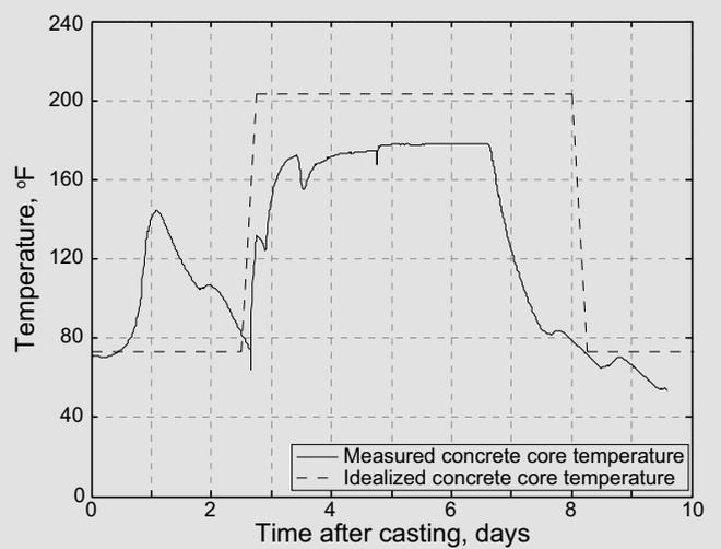
**Figure 9.** Core temperature of a 7.0 in. × 15 in. × 16.0 ft ultra-high-performance concrete beam during the curing of trial batch 4. Note: 1 in. = 25.4 mm; 1 ft = 0.305 m;  $^{\circ}\text{C} = (^{\circ}\text{F} - 32)/1.8$ .
