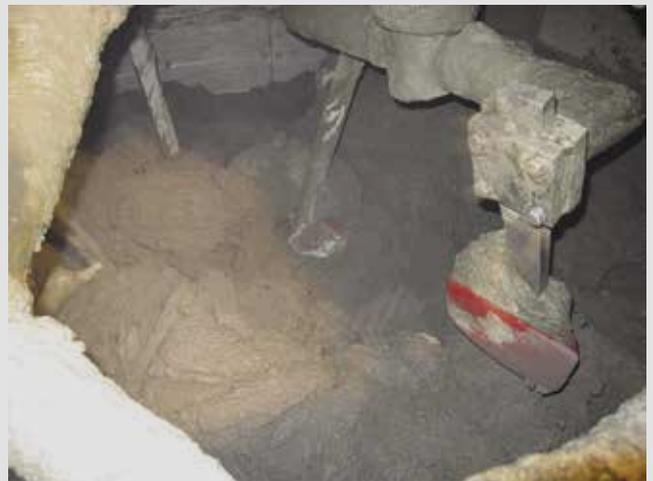
Desired consistency prior to fiber addition
