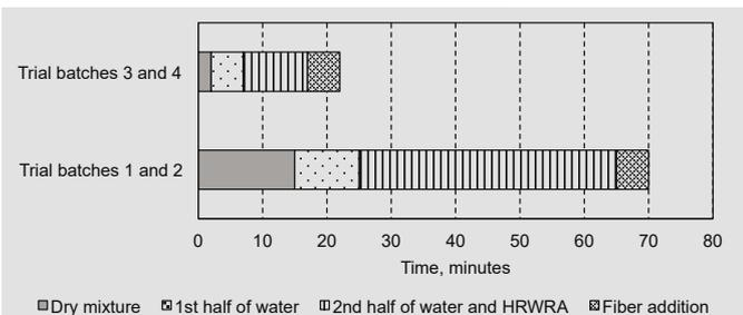
**Figure 2.** Average mixing times and procedures for the trial batches at the precast concrete plant.
