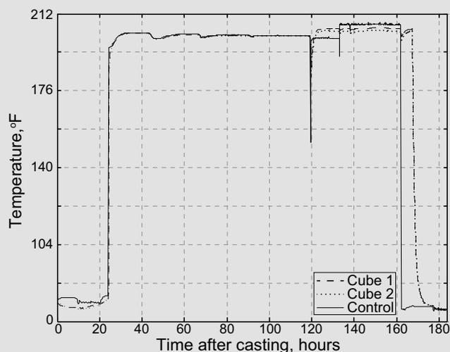
**Figure 1.** Typical core temperatures of a 4.0 in. ultra-high-performance concrete cube during the laboratory curing regimen. Note: 1 in. = 25.4 mm; °C = (°F – 32)/1.8.
