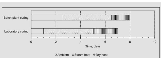
**Figure 3.** Comparison of batch plant and laboratory curing regimens.
