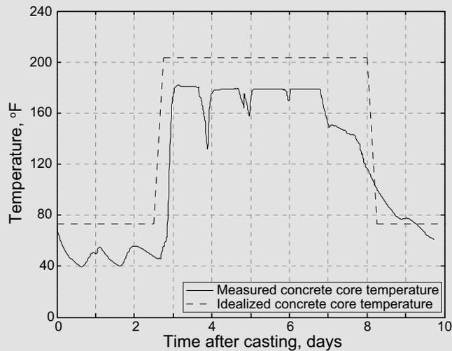
**Figure 8.** Core temperature of a 6.0 in. × 9.0 in. × 13 ft ultra-high-performance concrete beam during the curing of trial batch 3. Note: 1 in. = 25.4 mm; 1 ft = 0.305 m;  $^{\circ}\text{C} = (^{\circ}\text{F} - 32)/1.8$ .
