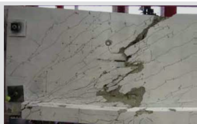
Figure 1. Precast concrete spandrel specimen tested at North Carolina State University. Image from Lucier et al., “Development of a Rational Design Methodology for Precast Concrete Slender Spandrel Beams: Part 1, Experimental Results” (2011).
