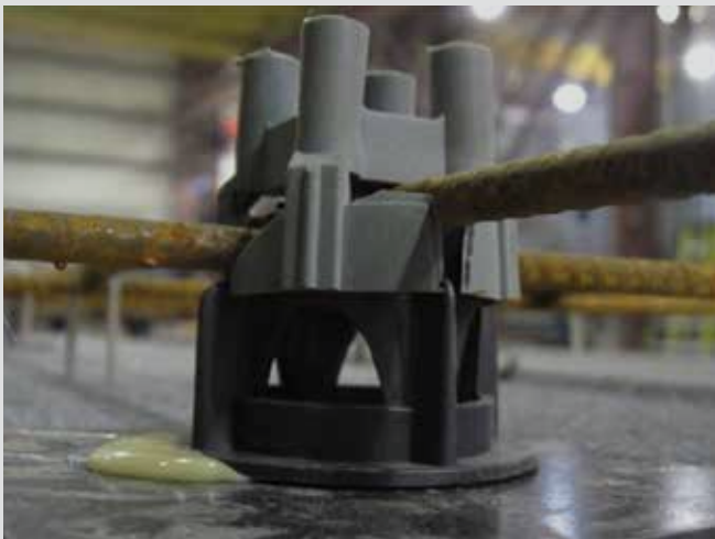
Structural wythe chair to reduce stress on foam during casting
