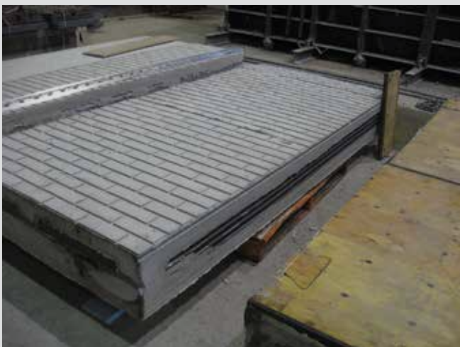
Final product with nonstructural architectural facade
