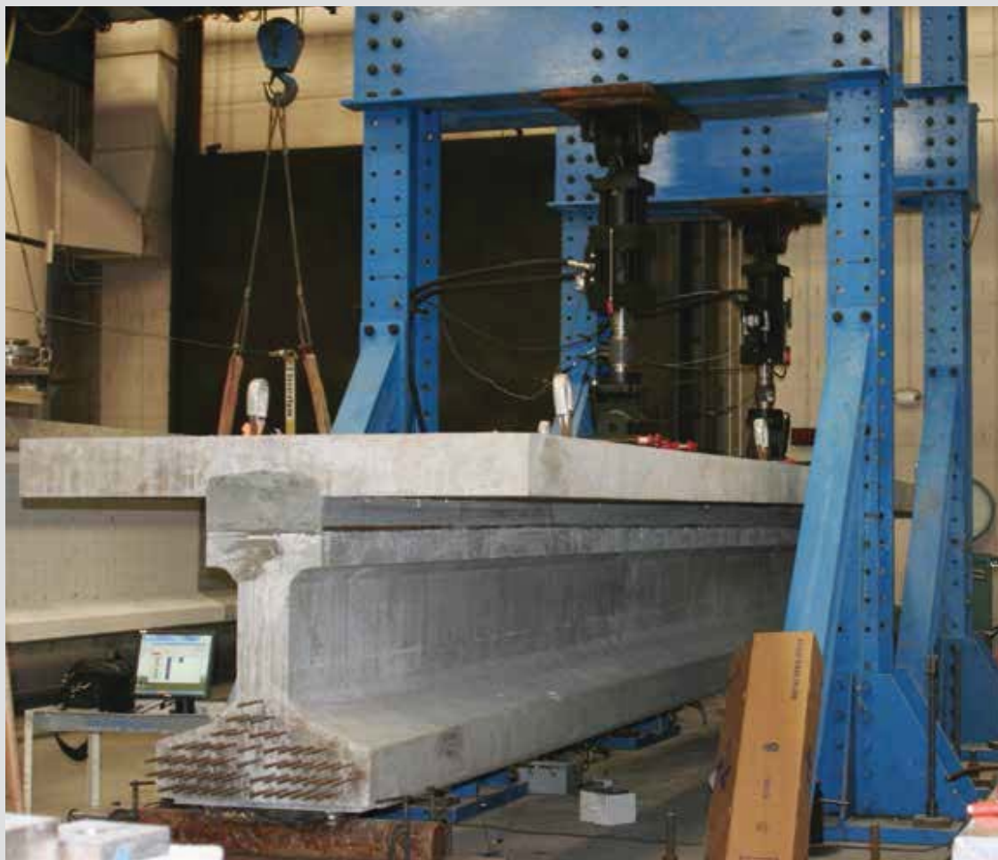
Figure 5. Test setup for cyclic loading of composite connection specimens.
