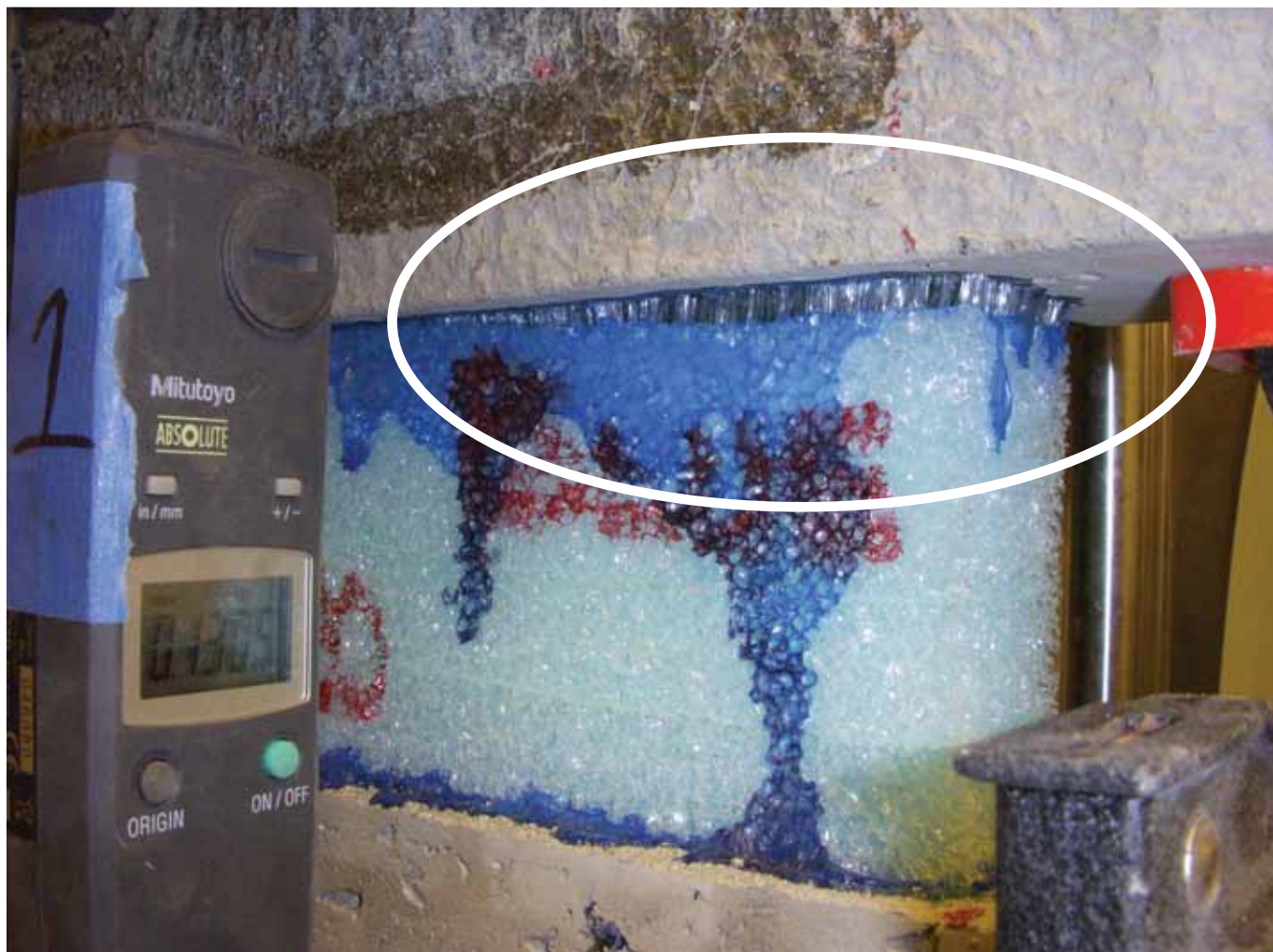
Figure 7. Failed specimen during tension test.
