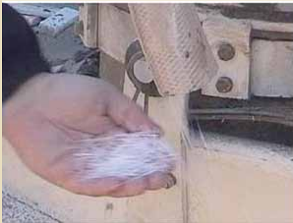
Figure 2. The new fiber-feeder system allows the feeding of discontinuous synthetic fibers to load-deflection curve in a mobile mixer. Photos courtesy of M. A. Issa, Mohammad A. Alhassan, and Jill Ramos.
