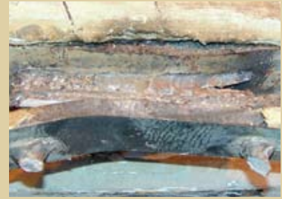
Figure 12. These diagrams and the photo show the plate flexural deformation from the plan view. Note: F_s = tension demand in bar; F_{sl} = tension demand in left bar; F_{sr} = tension demand in right bar; M_{nl} = moment demand in left bar; M_{nr} = moment demand in right bar; T = tension on slug weld.
