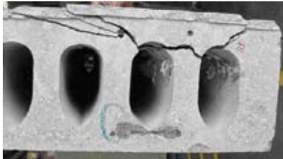
Fig. 3. Failure of base embed.
