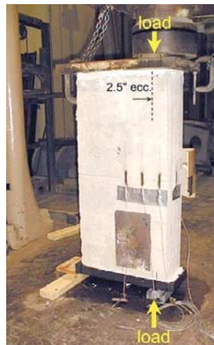
Fig. 16. Compression test prism with eccentric load.
