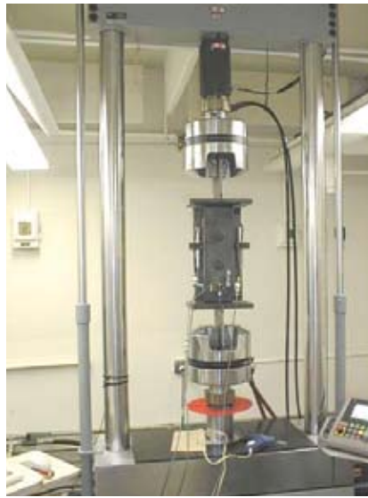
Fig. 19. Slotted-bolted connector test assembly in test machine.
