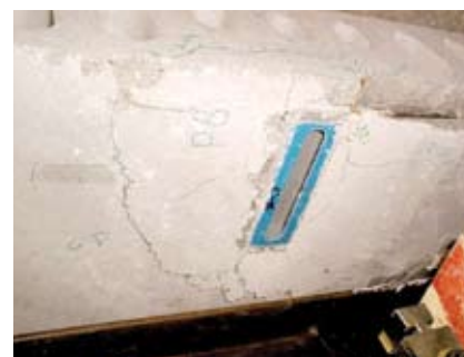
Fig. 12. Slotted connection tension test: flat failure surface.
