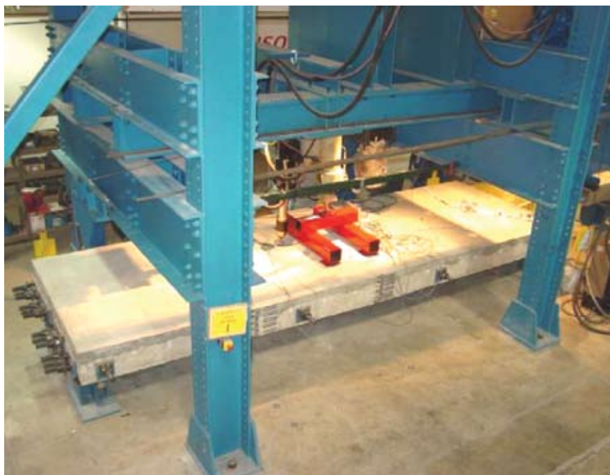
Fig. 10. Test setup of box-beam bridge models.
