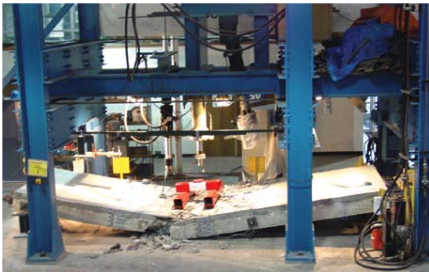
Fig. 11. Failure of bridge model BBD-I.
