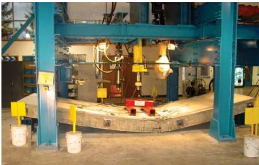
Fig. 12. Failure of bridge model BBD-II.
