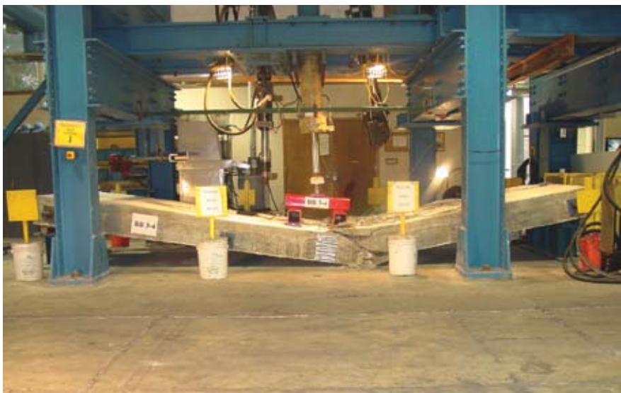
Fig. 13. Failure of bridge model BBD-III.
