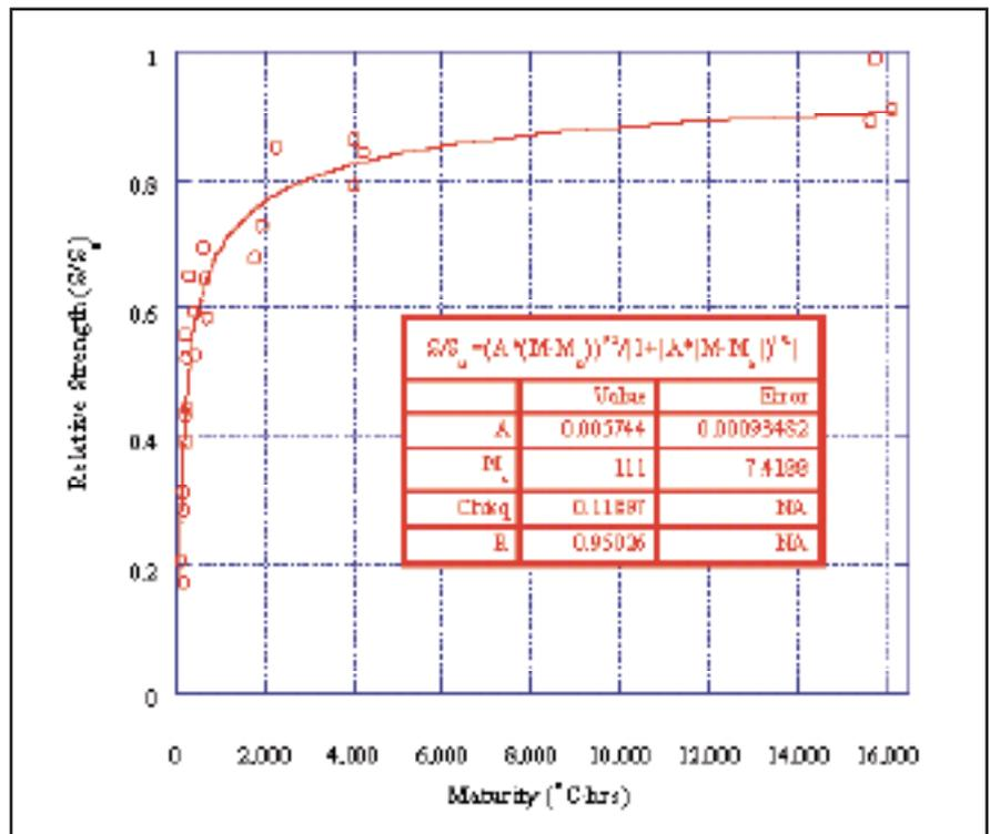
Fig. 9. Relative strength versus maturity for Mixture B, all trials.
