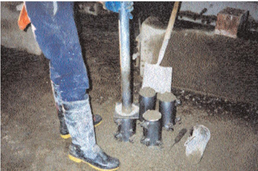
Fig. 2. Modified Proctor hammer used to compact zero-slump concrete into steel molds.
