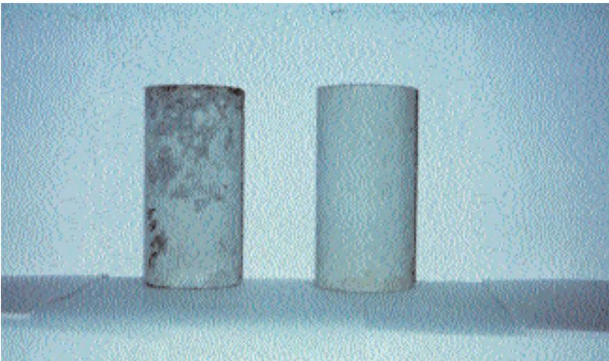
Fig. 3. On the left, a zero-slump test cylinder after stripping from the mold; on the right, a wet-cast test cylinder after stripping from the mold. Note the irregularity in appearance and voids in the zero-slump cylinder in comparison to the uniform appearance of the wet-cast cylinder.
