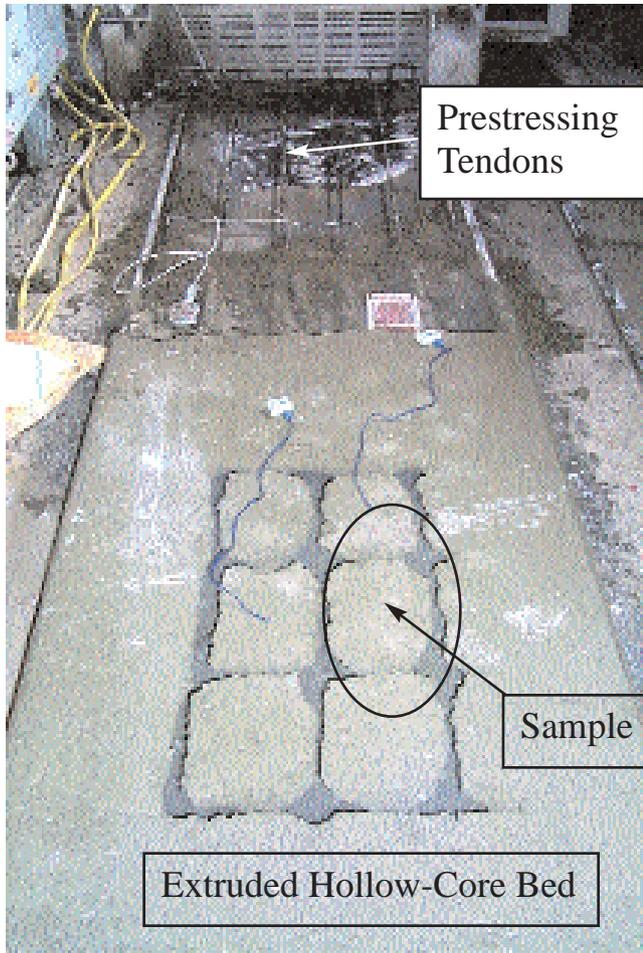
Fig. 5. Photograph of a typical sample: The top view shows chiseled samples on the bed; bottom left photo is an end view of a sample; and the bottom right shows a bottom view of a sample.
