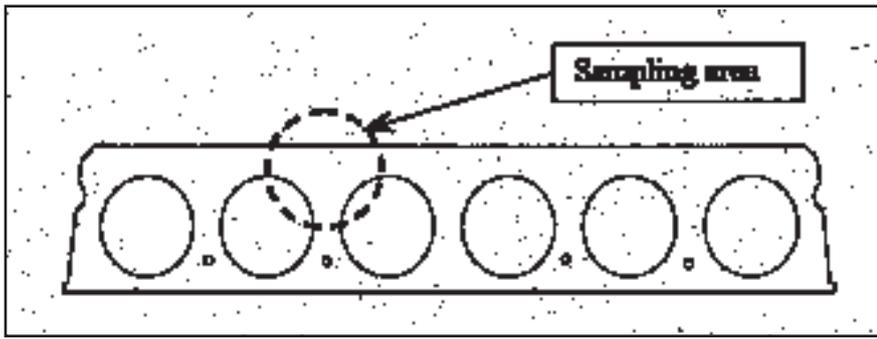
Fig. 4. Sampling area shown on typical hollow-core slab cross section.
