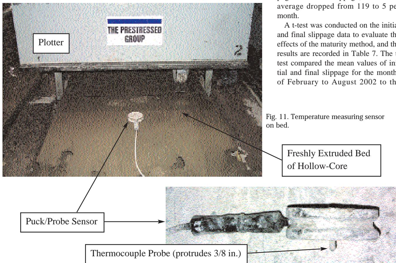
Fig. 11. Temperature measuring sensor on bed.
