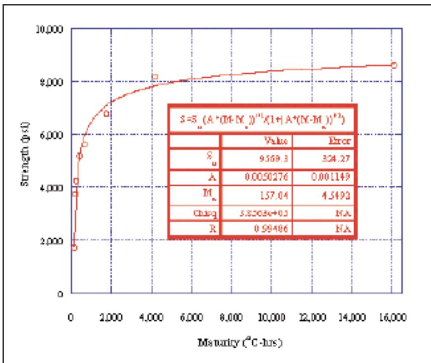
Fig. 8. Strength versus maturity for Mixture B, Trial No. 3.
