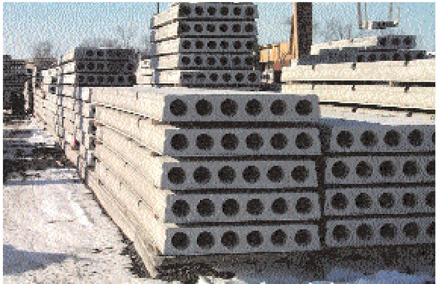
Fig. 1. Stacks of precast hollow-core concrete slabs in storage at PSI, Windsor, Ontario, Canada.
