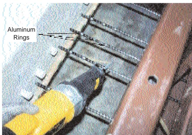
Fig. 4. Release of prestressing tendons with hand-held saw.
