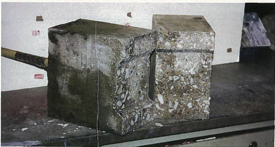
Fig. 5. Specimens for direct tension test.
