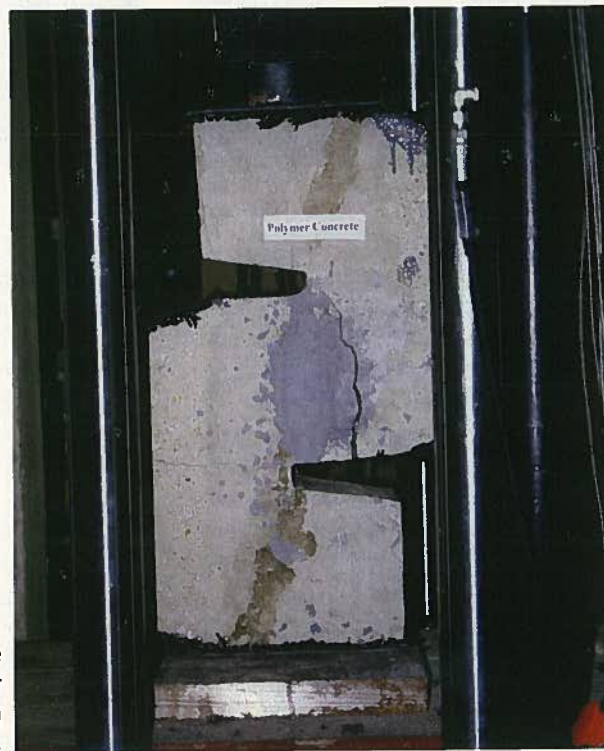
Fig. 10. Typical failure mode of vertical shear specimen cast with polymer concrete.
