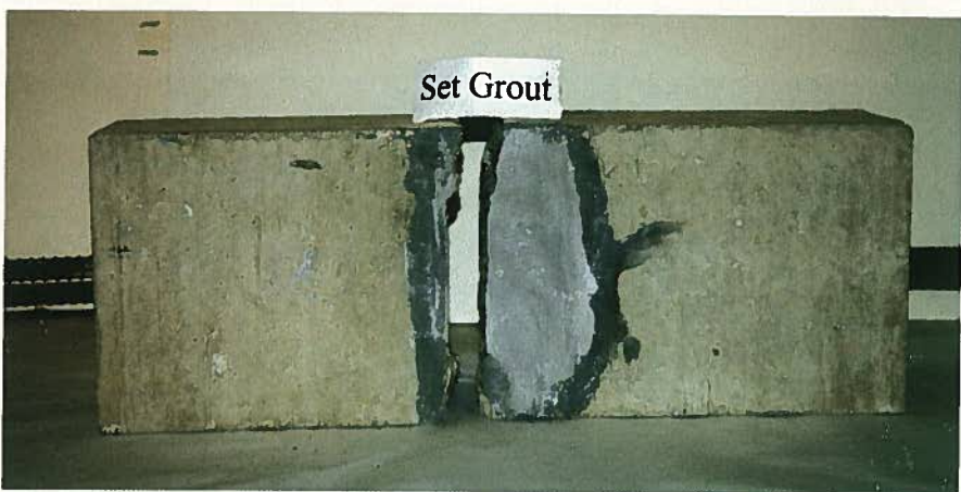
Fig. 12. Typical failure mode of direct tension specimen cast with Set Grout.
