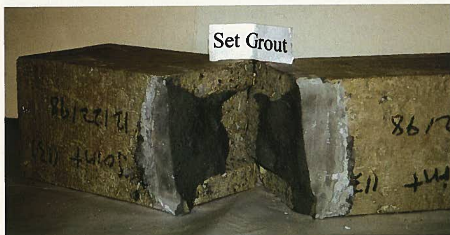
Fig. 15. Failure mode in Set Grout flexural specimen.
