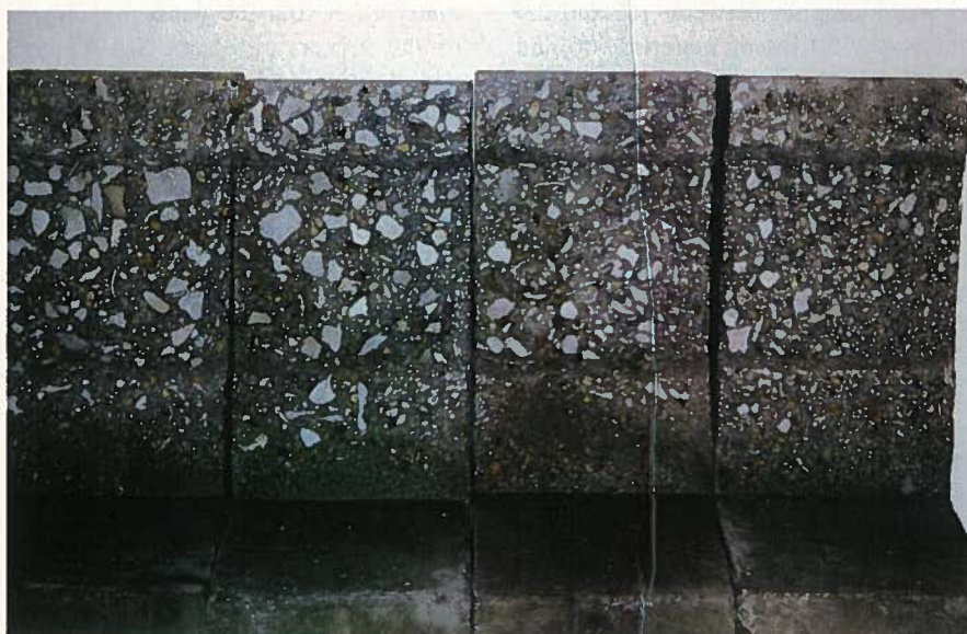
Fig. 6. Typical test specimens with sandblasted surface.
