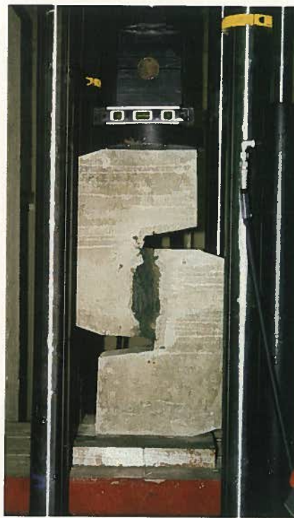
Fig. 7. Direct shear test setup.
