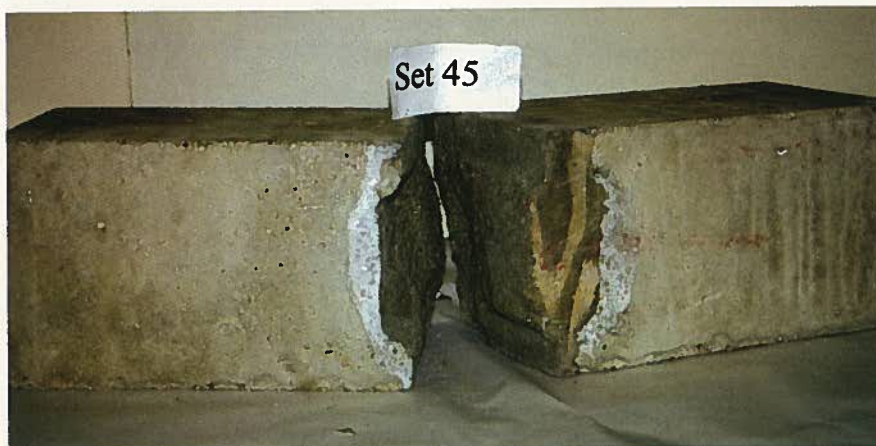
Fig. 14. Failure mode in Set 45 flexural specimen.
