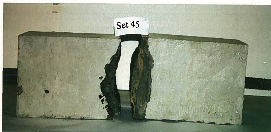
Fig. 11. Typical failure mode of direct tension specimen cast with Set 45.
