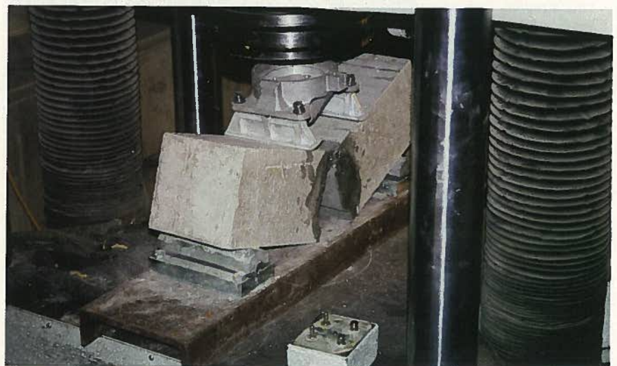
Fig. 9. Flexural testing setup.
