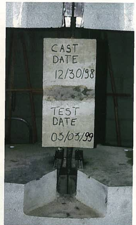
Fig. 8. Direct tension test setup.
