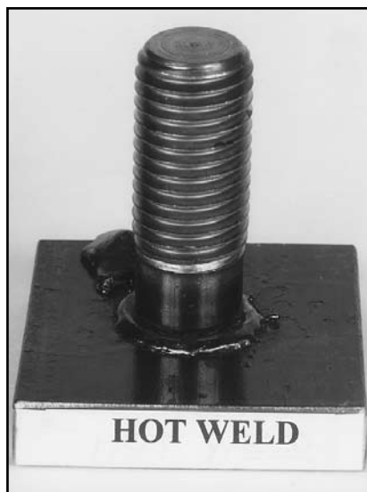
Fig. 12. Visual inspection of stud weld appearance. Source: Nelson Stud Welding, Inc.
