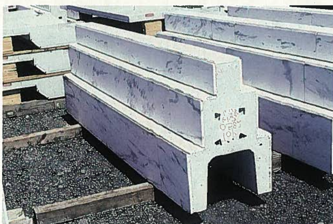
Fig. 17(b). Marble faced precast concrete fins are 3 x 6 ft (0.9 x 1.8 m) x variable length.
