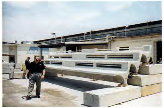
Fig. 9. Because of the uniqueness of the triple risers (Viñoly stadia) special load tests were carried out before mass production was initiated. These tests proved to be satisfactory.
