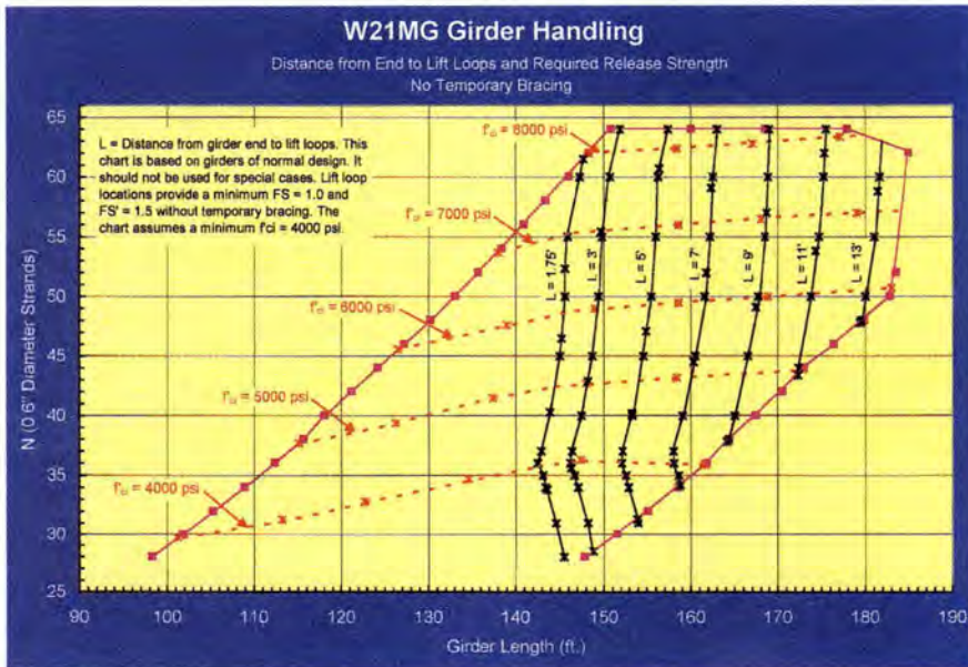
Fig. 21. W21MG girder handling without bracing.
