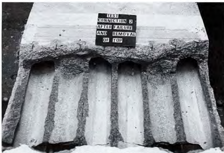
Fig. 19. The end of Test B on connection Type 2 (top view of end of unit).
