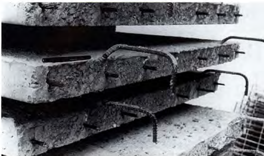
Fig. 2. Example of hanger bars for precast concrete floor units used in New Zealand.
