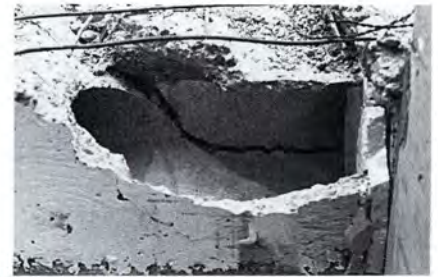
Fig. 16. The end of Test A on connection Type 2 (side view of end of unit).
