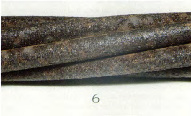
Photo 6. Strand surface before cleaning.
