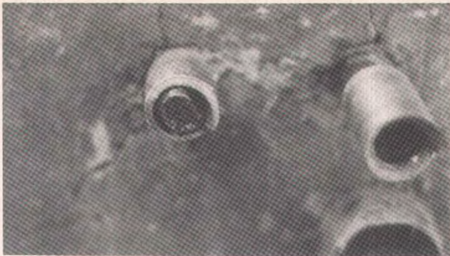
Fig. 3. Specimen BC99 — top couplers at failure.
