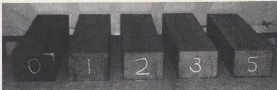
Fig. 63. Freeze-thaw test specimens of epoxy mortar with different moisture content.
