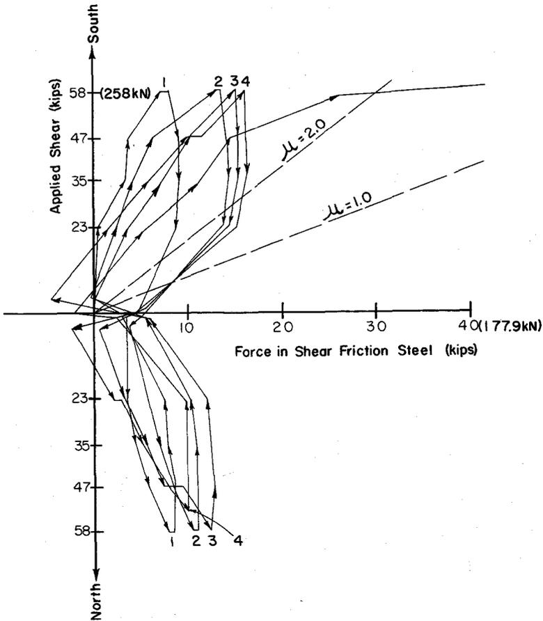
Fig. 8. Applied shear vs. force in shear-friction steel.
