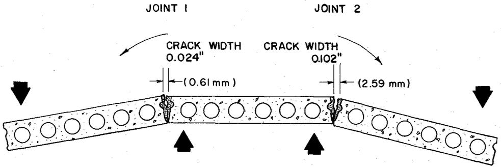
Fig. 6. Artificial cracking of joints.
