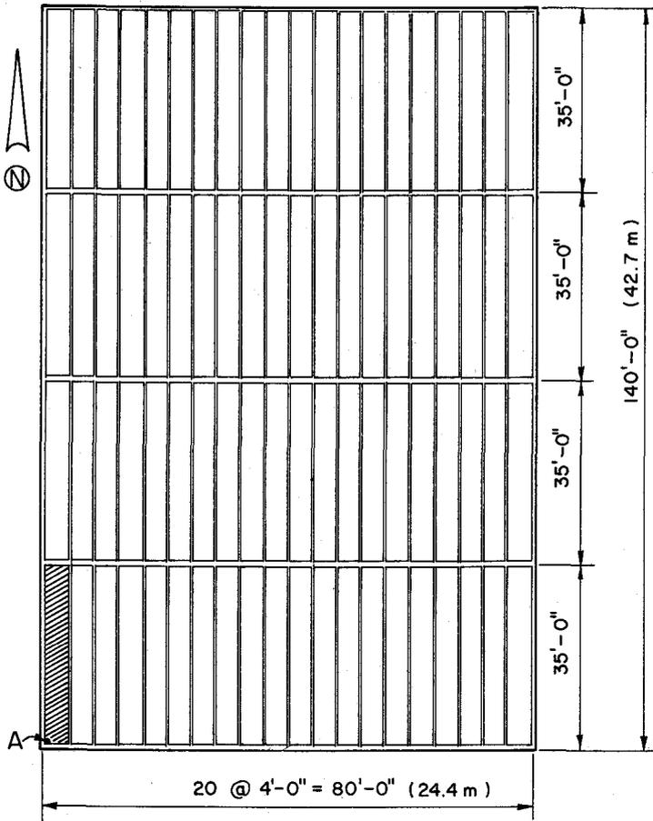
Fig. 1a. Floor plan used in numerical example.
