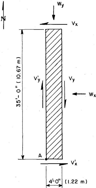
Fig. 1b. Free body diagram of panel (Section A) shown in Fig. 1a.
