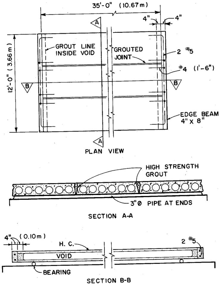
Fig. 3. Assembly of test specimens.
