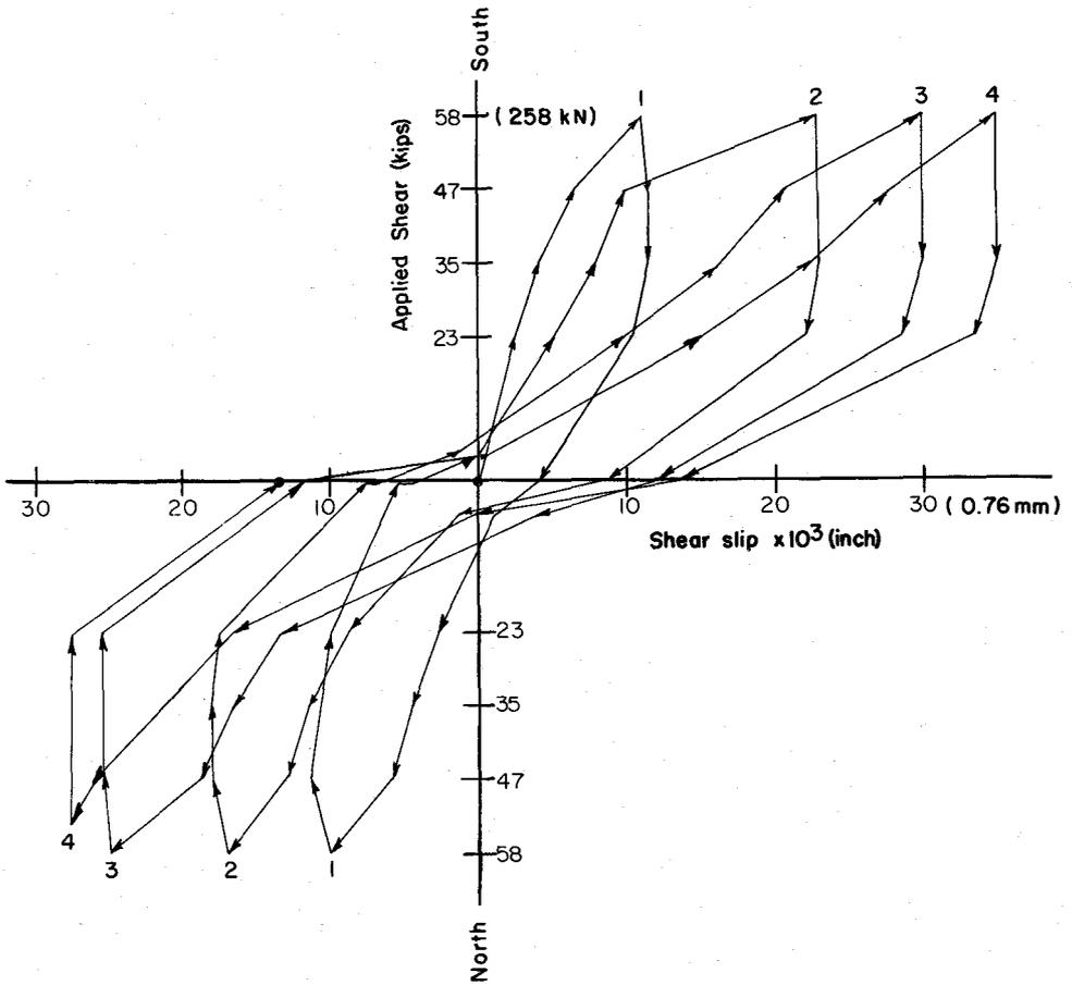
Fig. 9. Relationship between applied shear and shear slip along the joint.
