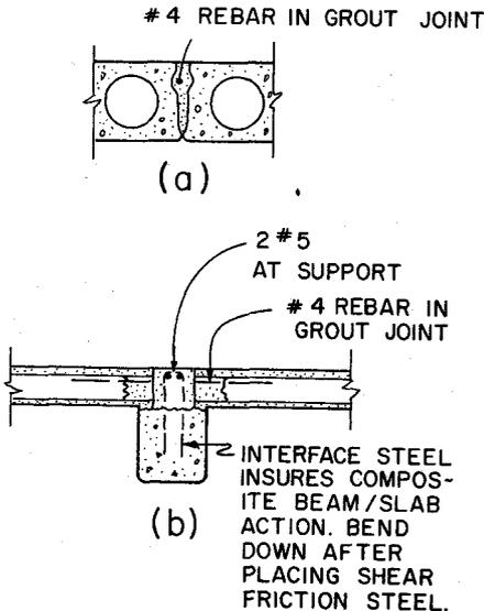
Fig. 2. Shear-friction reinforcement details.
