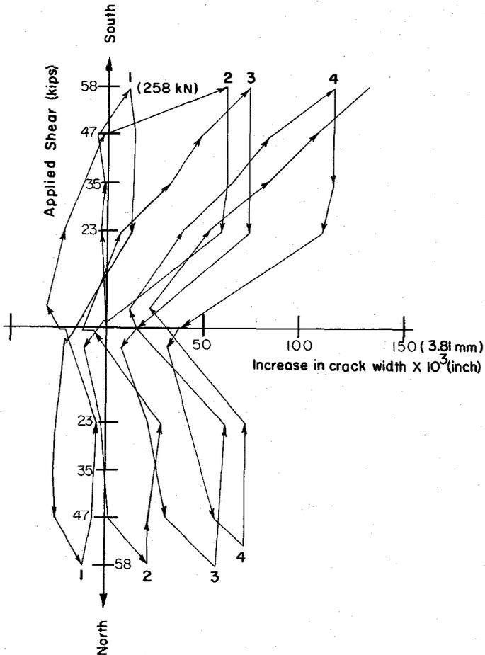
Fig. 7. Applied shear vs. increase in crack width.
