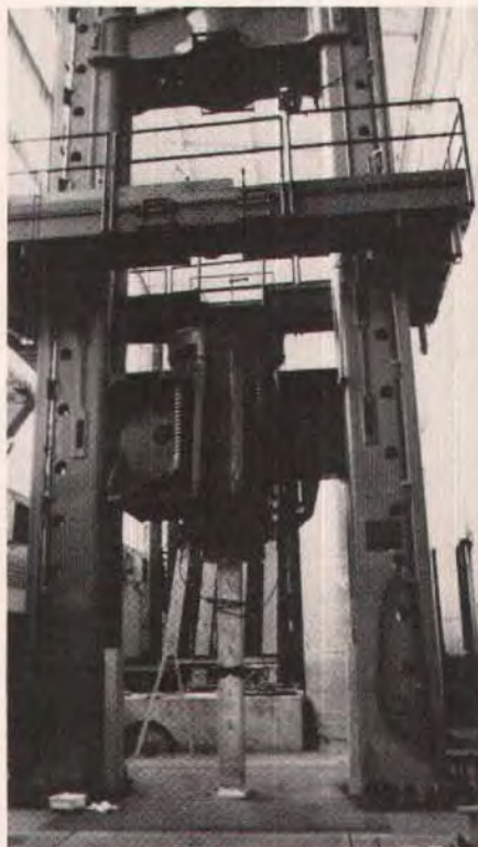
Fig. 20. Arrangement for testing of compression specimens.
