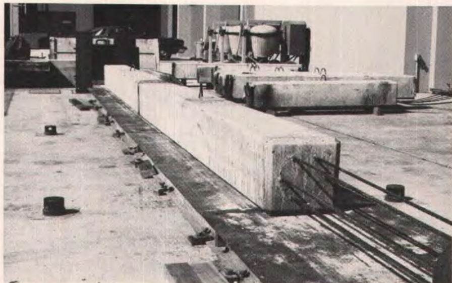
Fig. 8. Test bed for tension testing.
