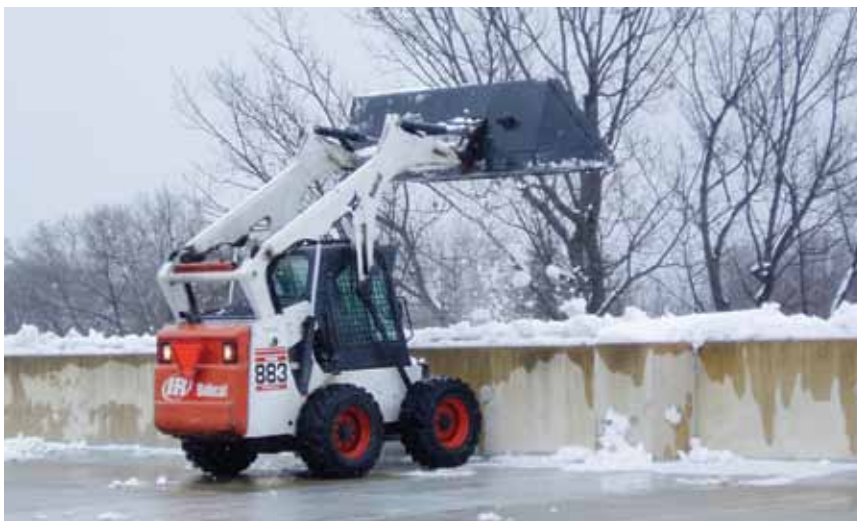
Designers should discuss snow and ice removal with the owner to determine if any snow-storage areas, dump zones with snow gates or special admixtures or waterproofing details should be provided.
