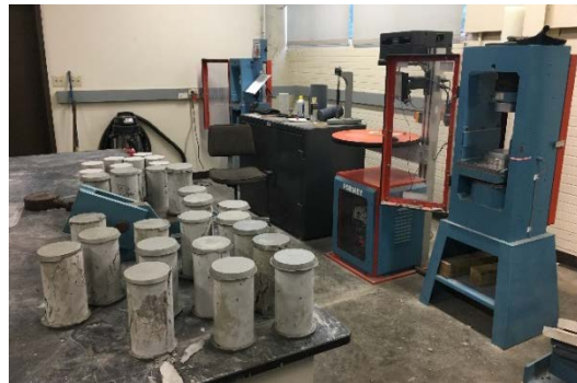
(f) Periodic testing of match-cured cylinders
