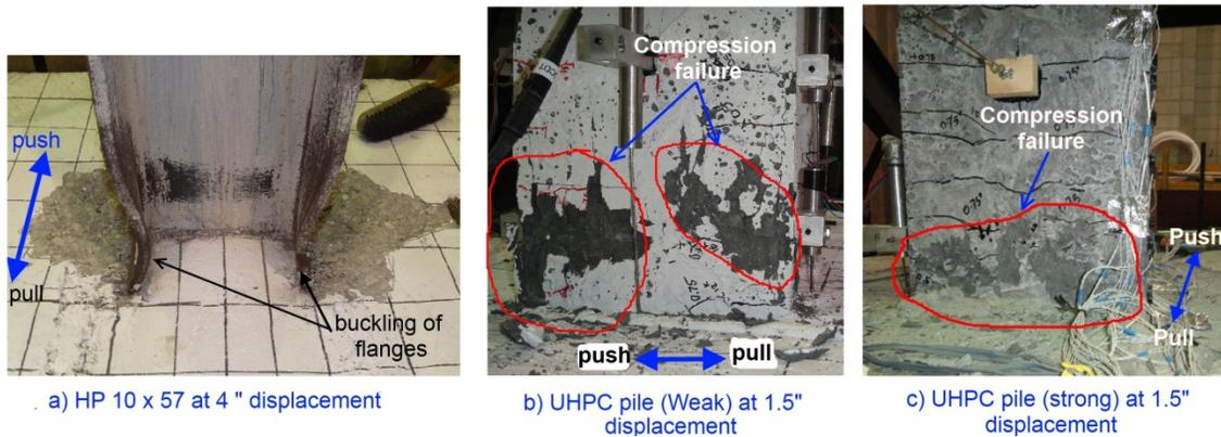
Figure 11 Observed damage to piles and abutment at failure
