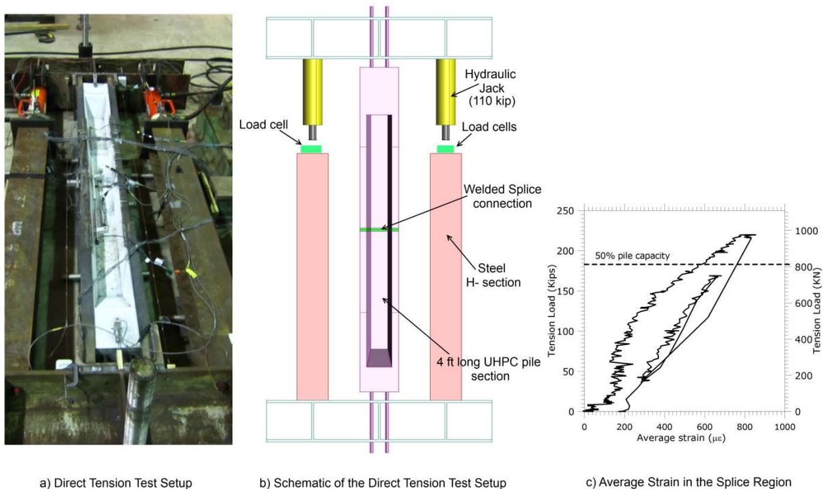
**Figure 5 Direct tension setup and observed splice behavior**
