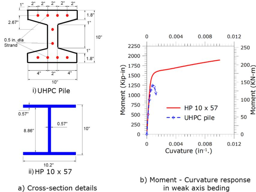
**Figure 1 Comparison of details and section behavior of UHPC pile and steel HP 10x 57**
