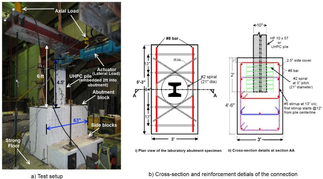
**Figure 8 Test setup and the pile-to-abutment connection details**
