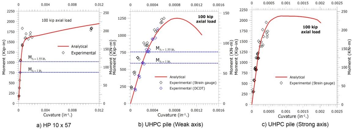
Figure 10 comparison of measured and calculated moment curvature response for steel and UHPC piles
