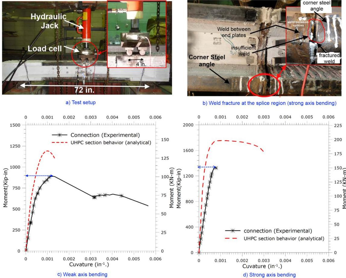
**Figure 7 flexural Test setup and observed moment-curvature response of splice region in weak and strong axis directions**
