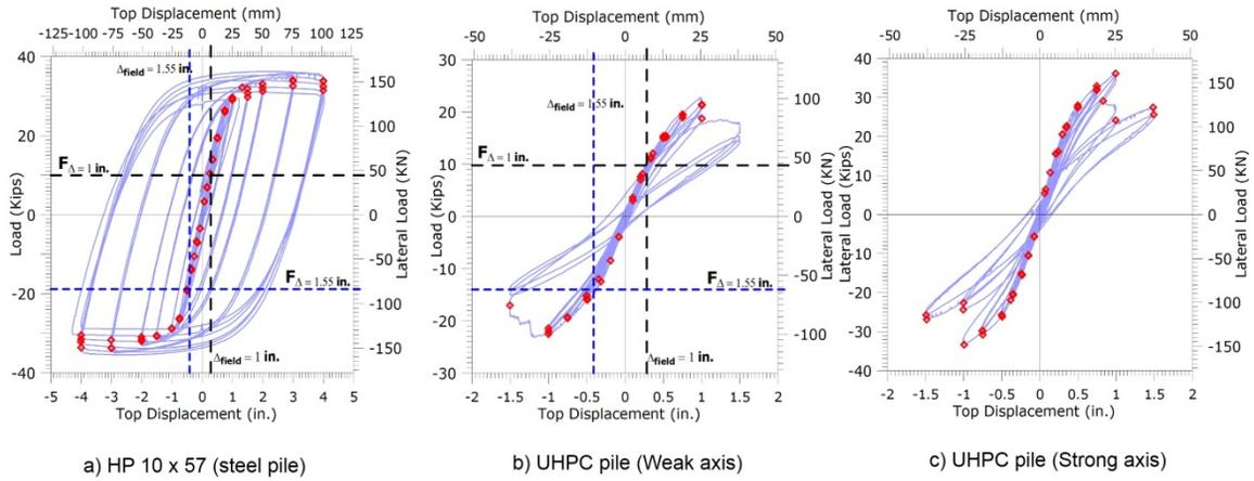
Figure 9 Measured force-displacement response of steel and UHPC piles
