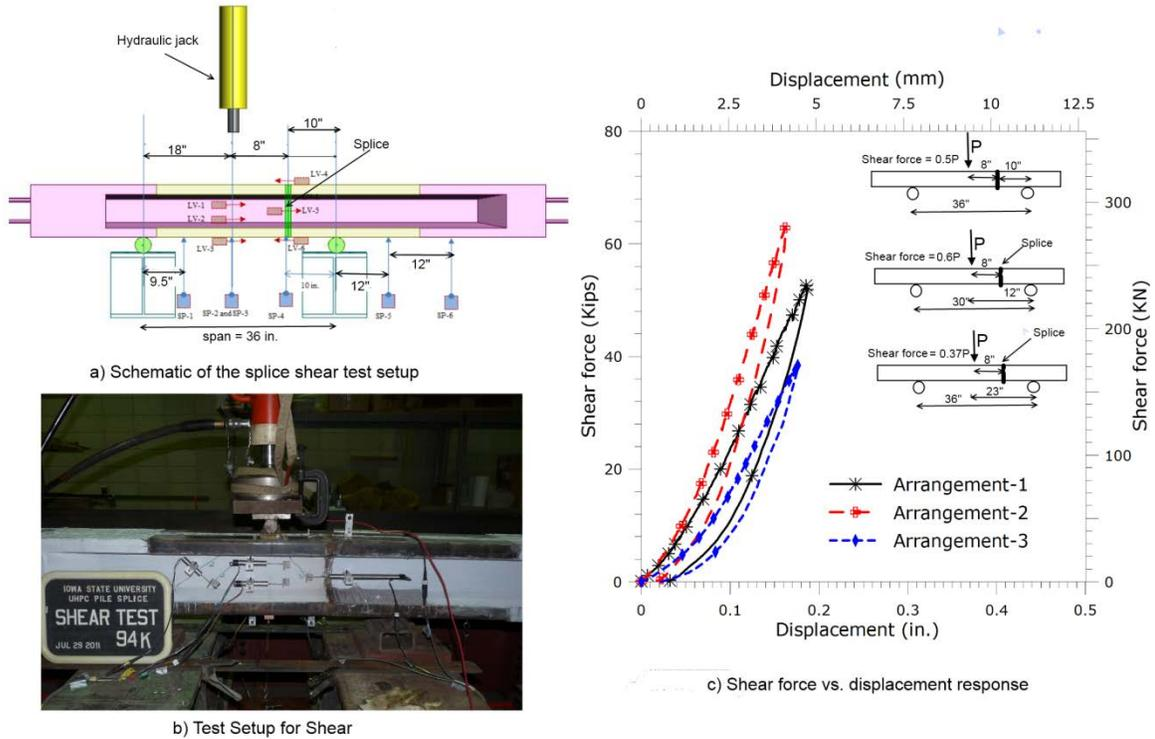
Figure 6 Shear test setup and observed shear force vs. displacement behavior.
