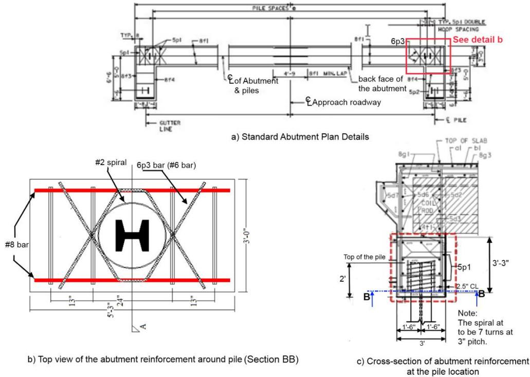
**Figure 4 Standard pile-to-abutment connection details used in Iowa**
