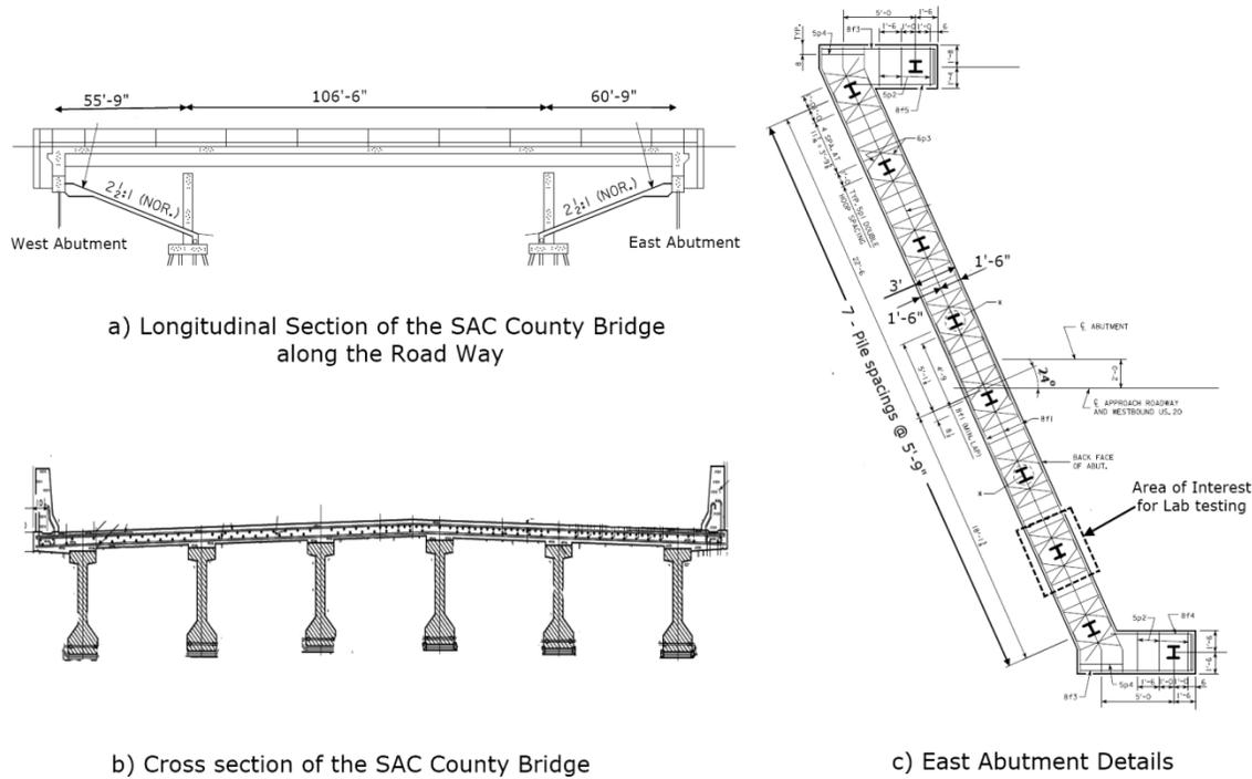
**Figure 2 Details of the SAC County Bridge in Iowa**
