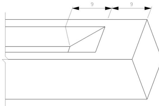
Fig. 7 Recommended expanded region at top of UHPC pile to minimize driving stresses
