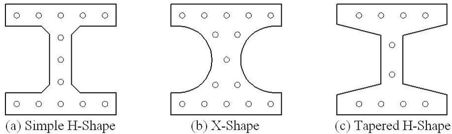
Fig. 3 Different H-shaped sections investigated for UHPC piles
