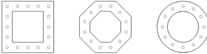
Fig. 2 Hollow prestressed UHPC sections initially considered in the study
