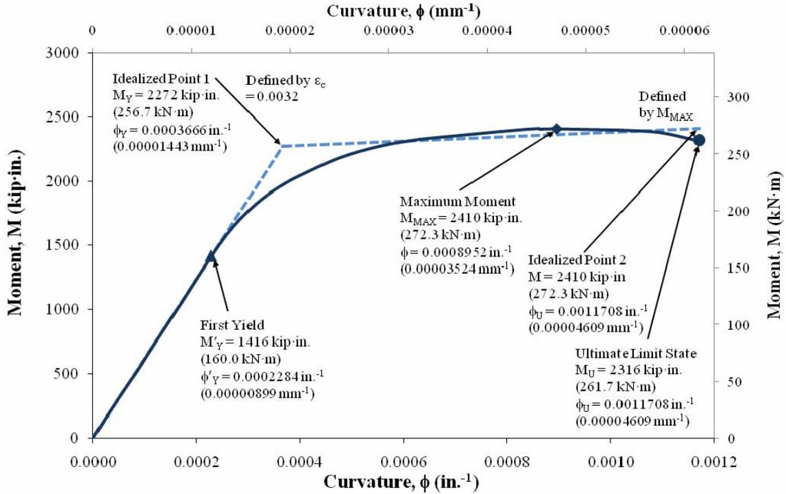
Fig. 5 Moment-curvature idealization for UHPC pile with 200 kip (890 kN) axial load (if you can, label the actual response and idealized response in the figure)
