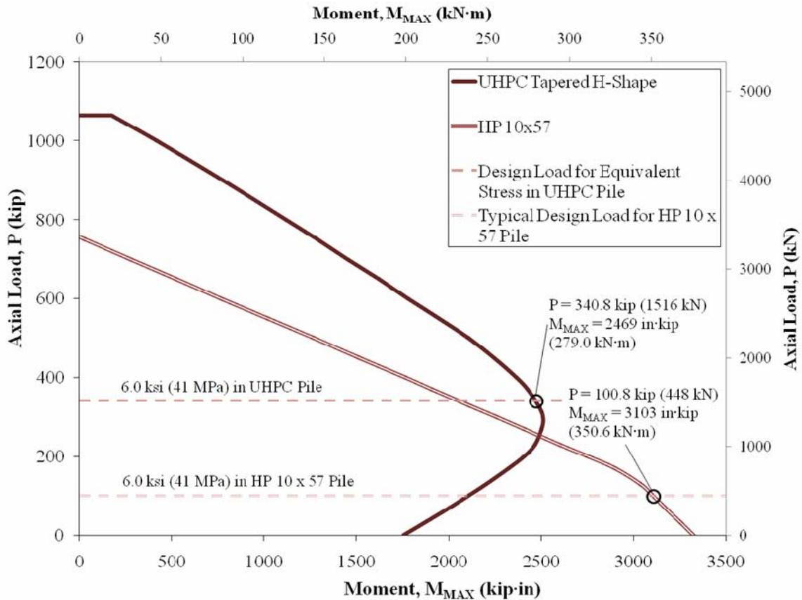
Fig. 6 Interaction diagram developed for the maximum moment resistance of a tapered H-shaped UHPC and a HP 10 x 57 steel section
