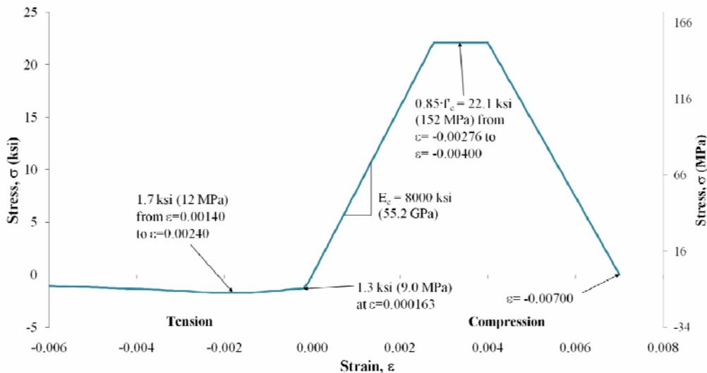
Fig. 1 Stress-strain behavior for UHPC
