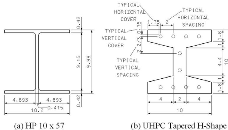
Fig. 4 Dimensions of comparable steel and UHPC pile sections
