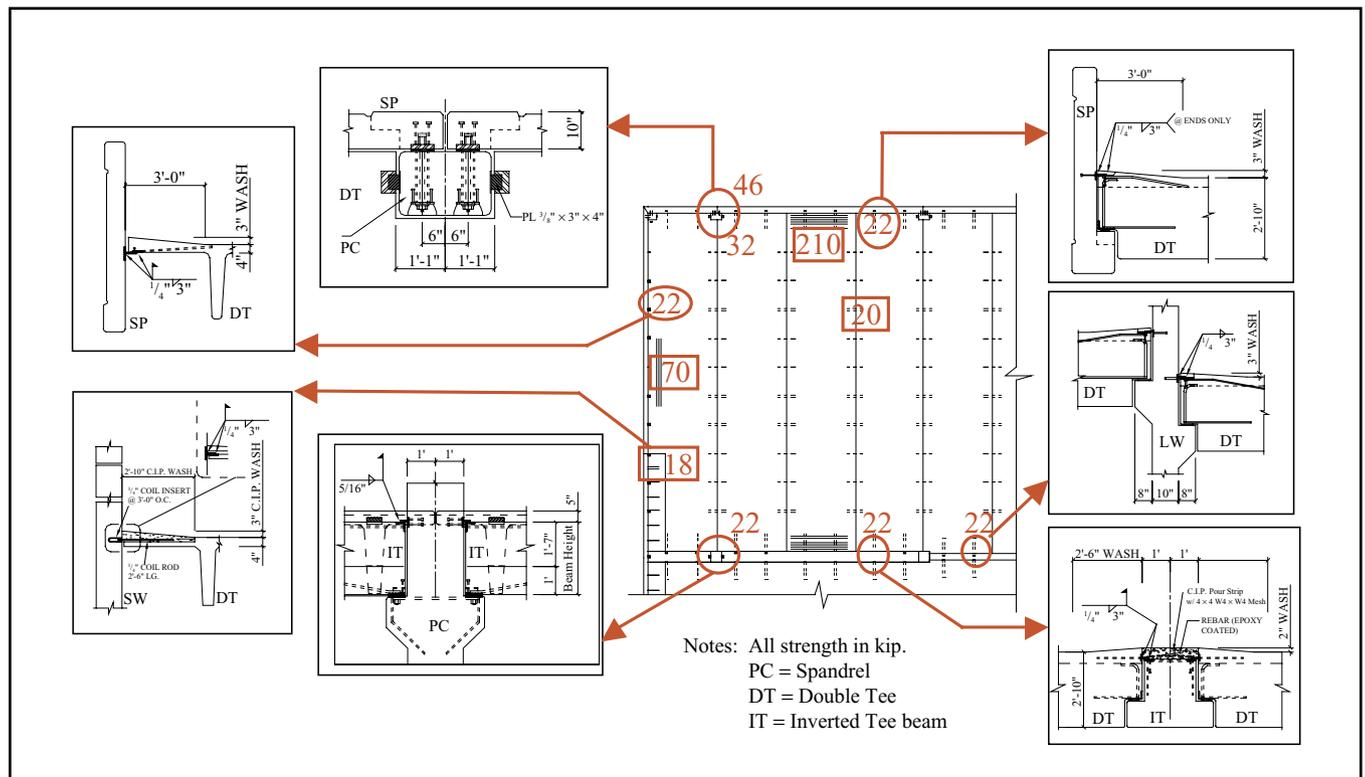
Fig. 3. Diaphragm secondary details. Note: 1 in. = 25.4 mm; 1 kip = 4.448 kN; 1 ft = 0.3048 m.
