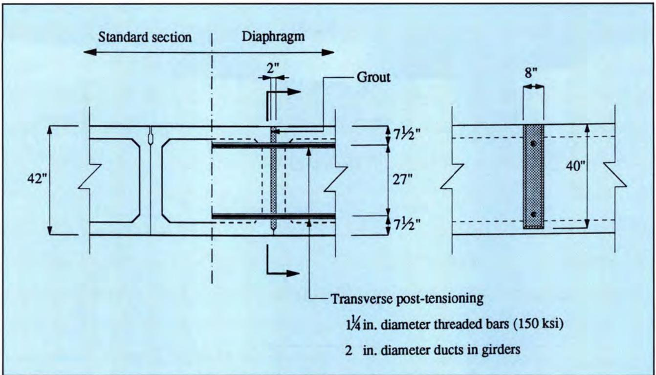
Fig. A5. Transverse post-tensioning arrangement. **Note:** 1 in. = 25.4 mm; 1 ksi = 6.895 MPa.
