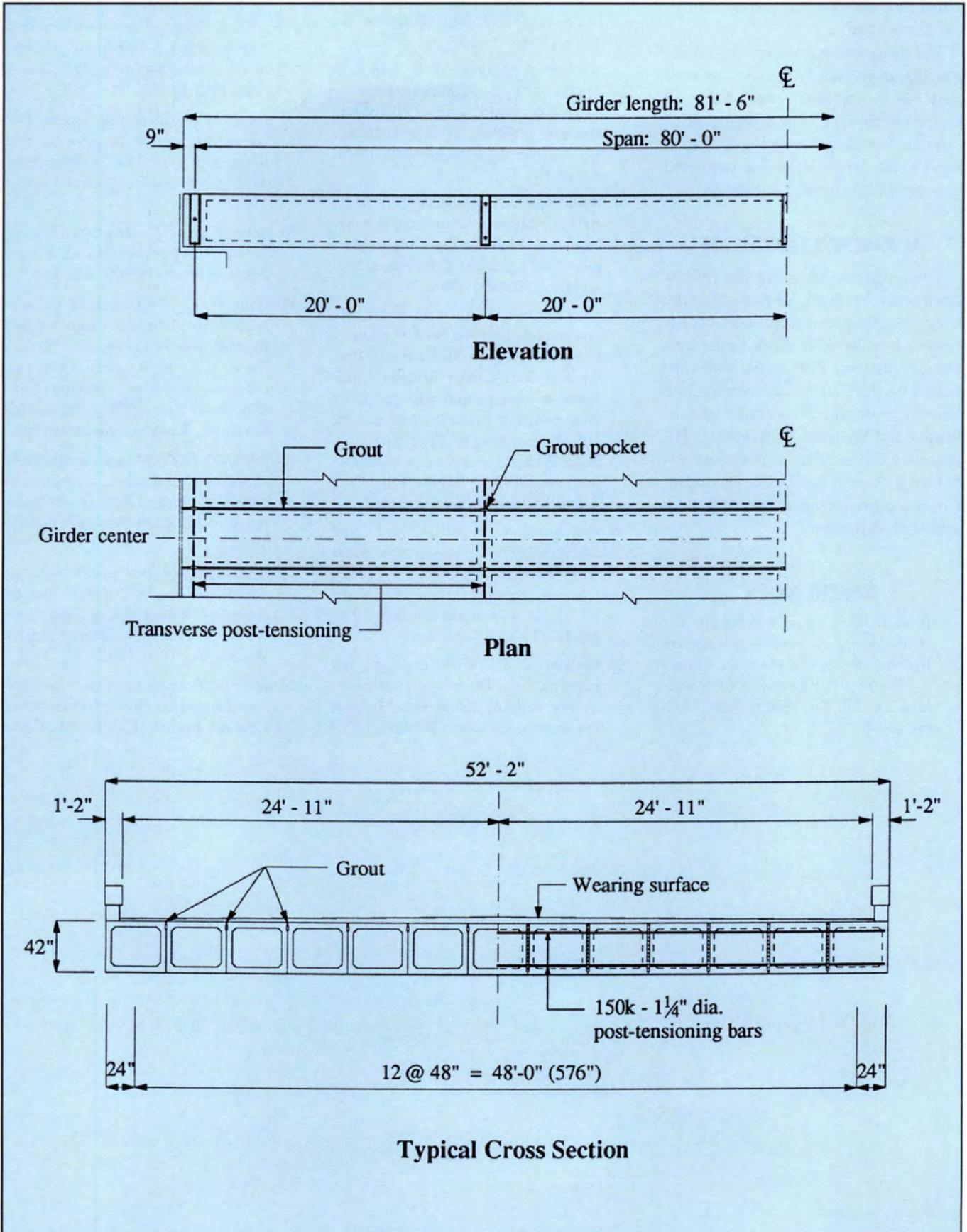
Fig. A1. General view of bridge for proposed design. **Note:** 1 in. = 25.4 mm; 1 ft = 0.305 m.
