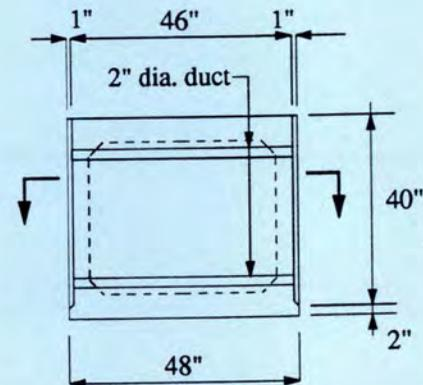
Modified Precast Section at Diaphragm
