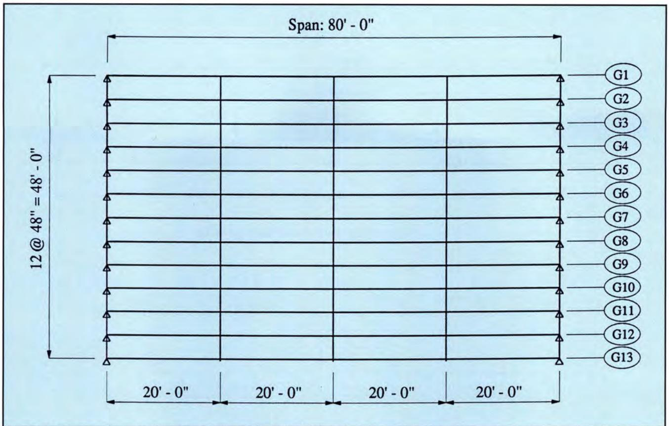
Fig. A2. Model of grid analysis. **Note:** 1 ft = 0.305 m.
