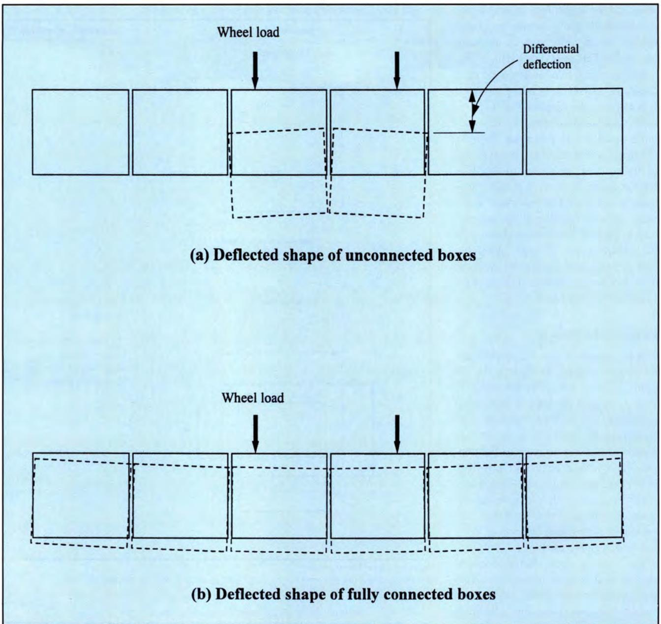
Fig. 8. Schematic of deflected shape of box girder bridge.
