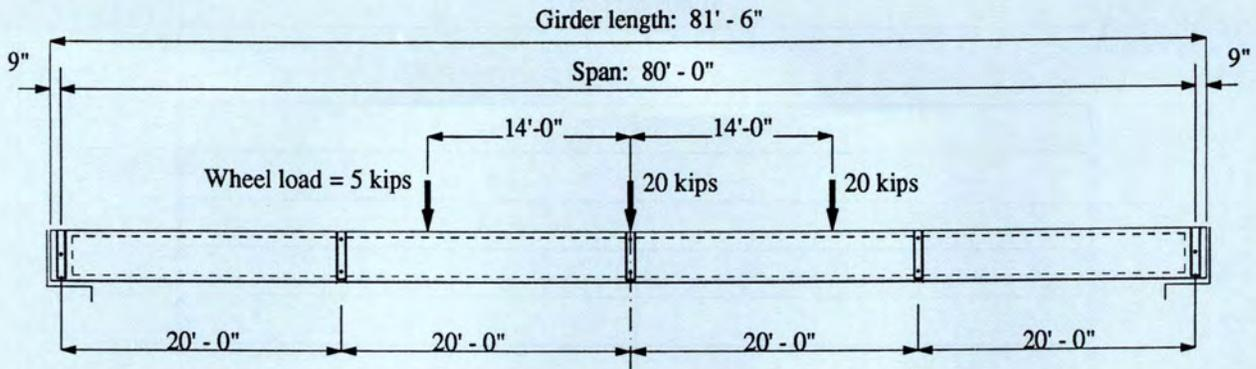
(a) Elevation and wheel load position
