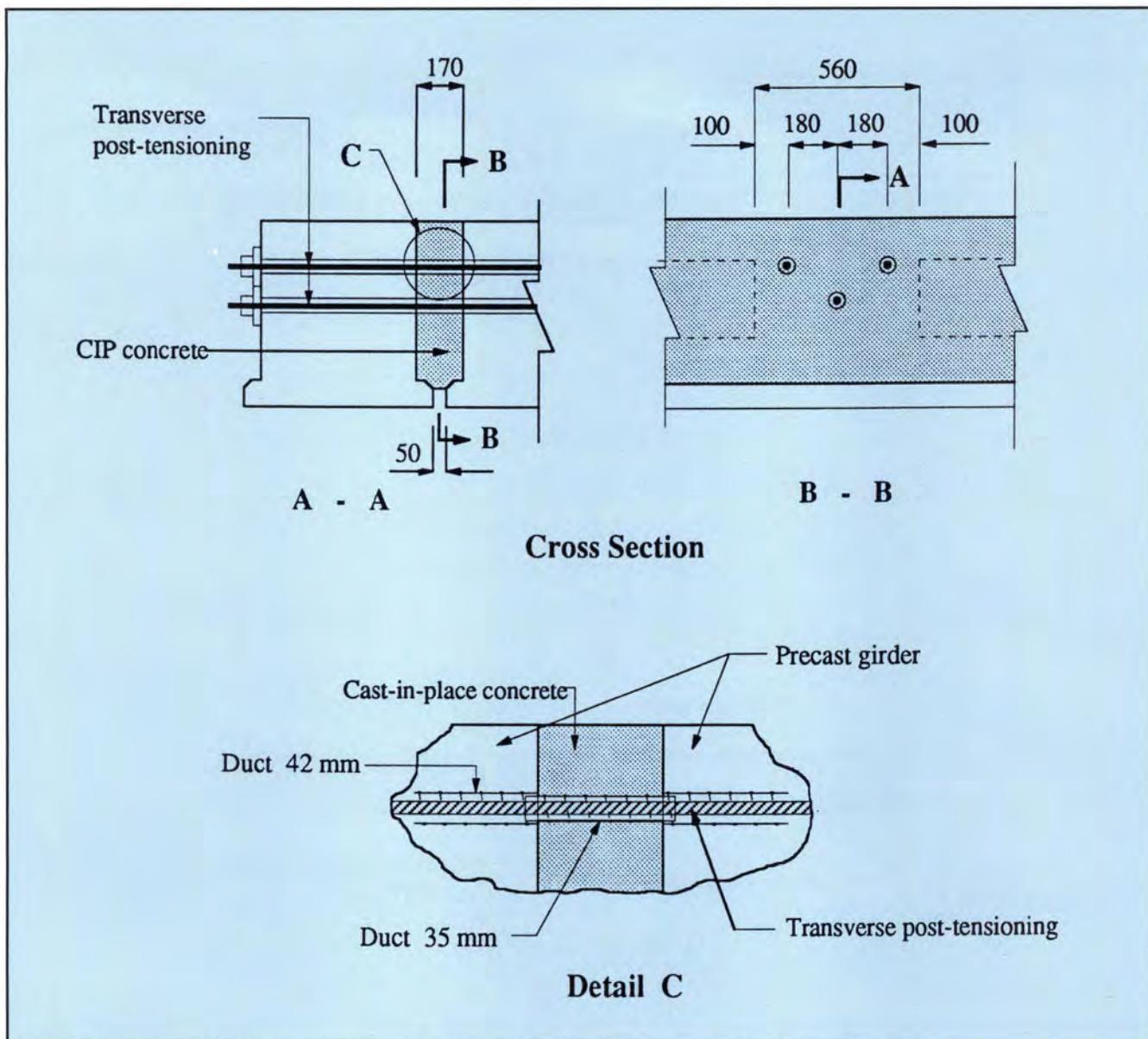
Fig. 4. Transverse post-tensioning arrangement for Japanese box girder bridges. Dimensions are in millimeters.
