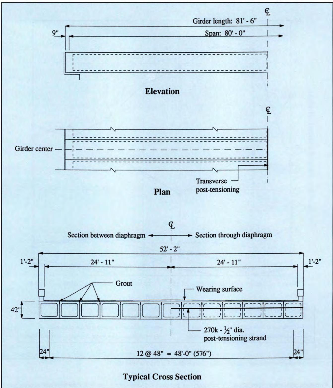
Fig. 2. Elevation, plan and typical cross section of precast box girder bridges in the United States. **Note:** 1 ft = 0.305 m; 1 in. = 25.4 mm.
