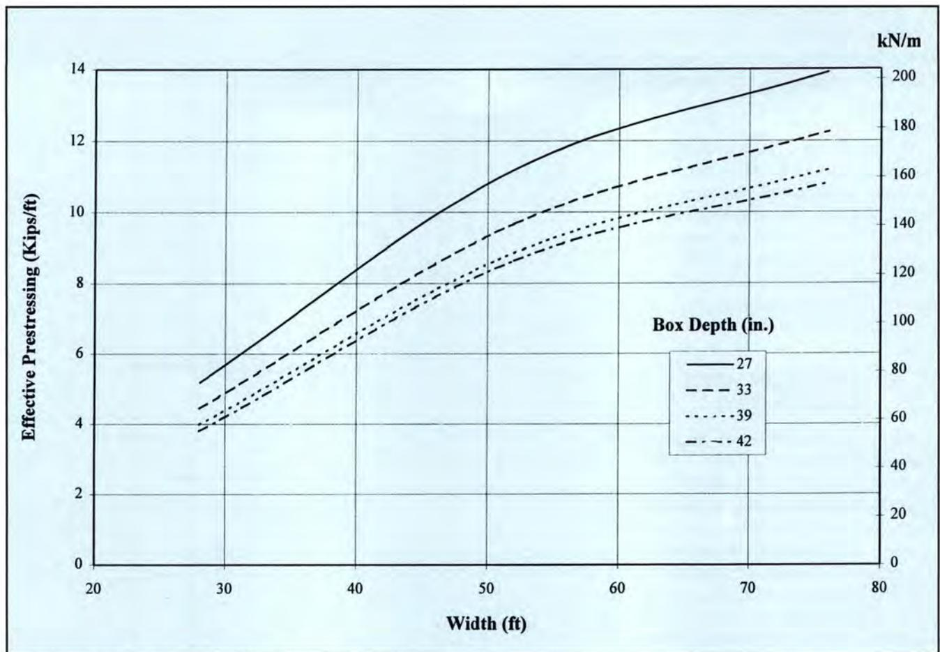
Fig. 10. Prestressing force for midspan diaphragm. **Note:** 1 ft = 0.305 m.
