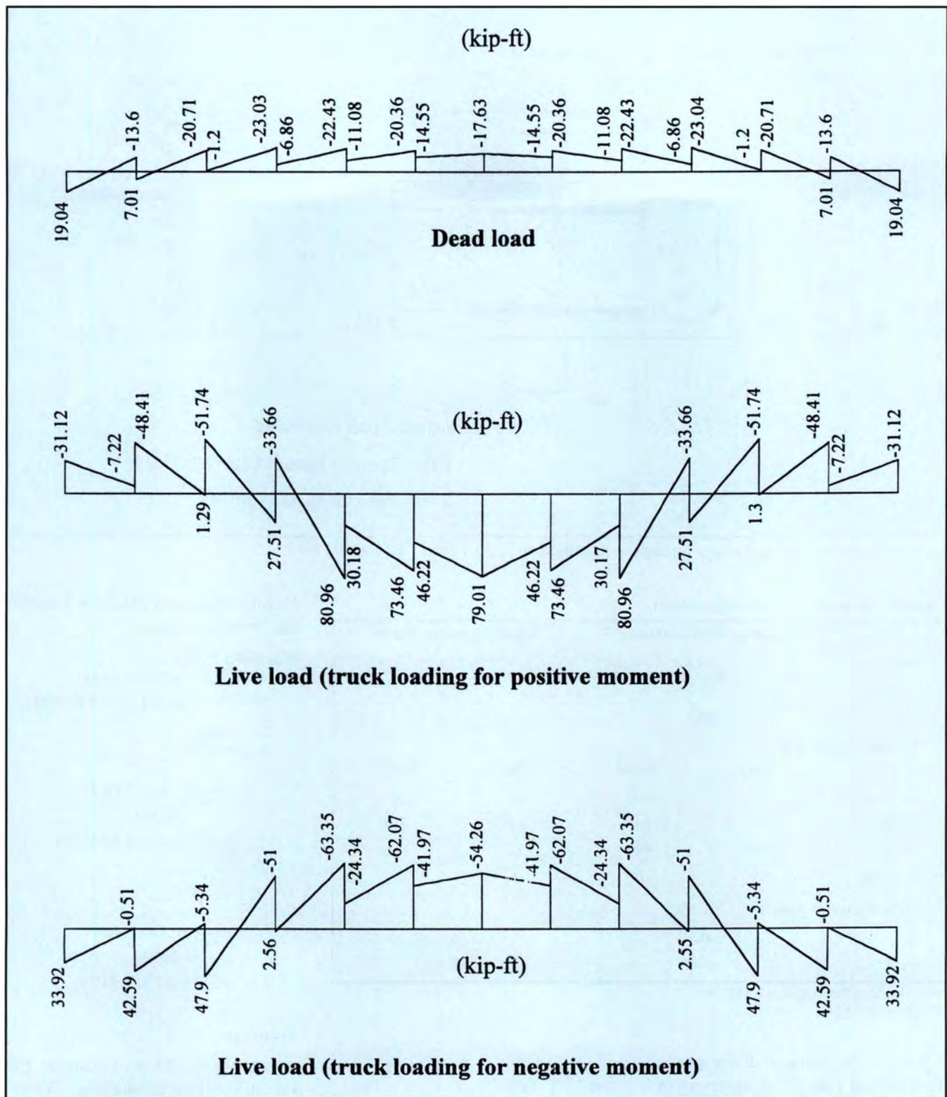
Fig. A4. Moment diagram in midspan diaphragm due to truck loading. **Note:** 1 kip-ft = 1.356 kN-m.
