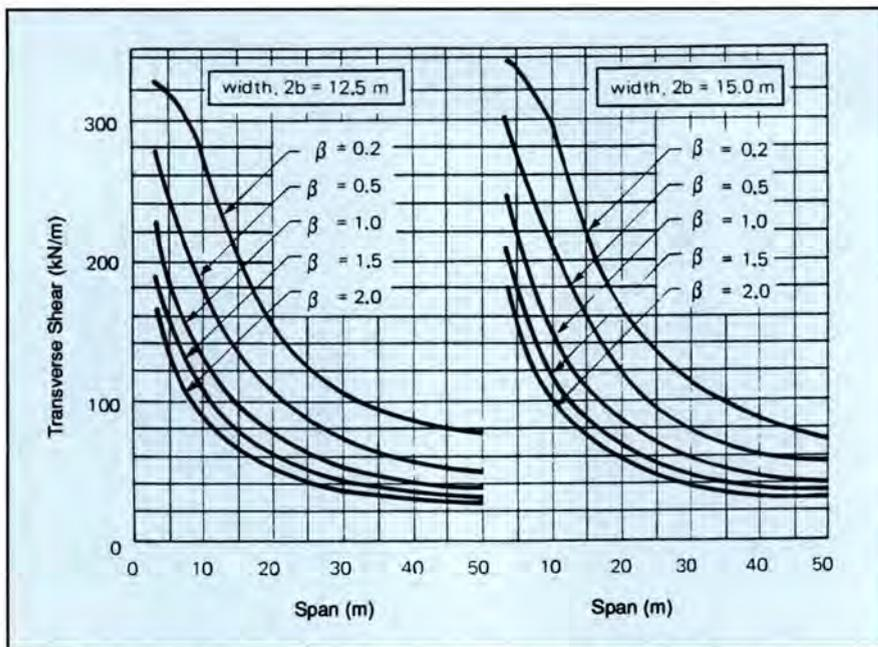
Fig. 7. Ontario Code design chart (Ref. 4). Note: 1 kN/m = 0.0685 kips per ft; 1 m = 3.28 ft.
