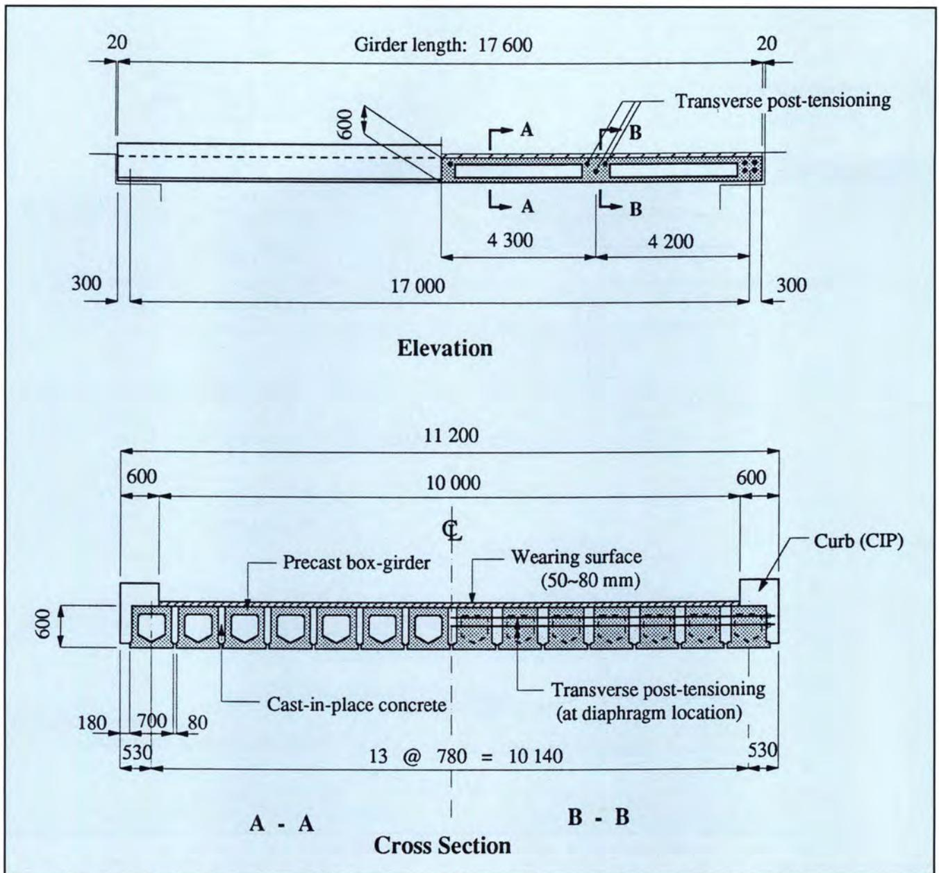
Fig. 3. Precast, pretensioned concrete box girder bridge system for simple short span. **Note:** 1 m = 3.28 ft; 100 mm = 3.94 in.
