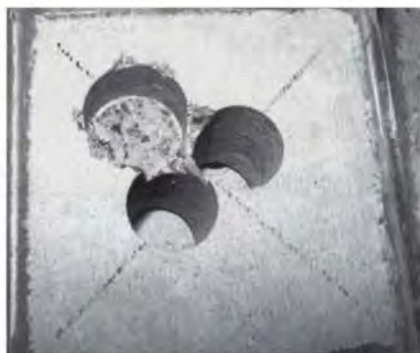
Fig. 1. Slab after coring to remove chloride samples.
