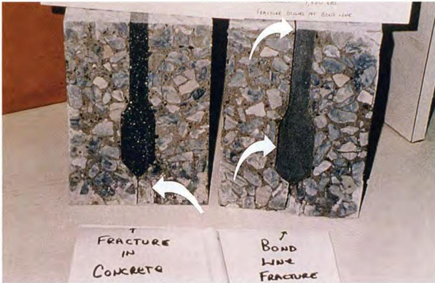
Fig. 11. Comparative failure modes: vertical shear composite tests.
