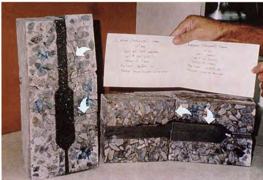
Fig. 12. Comparative failure modes: longitudinal composite shear tests.
