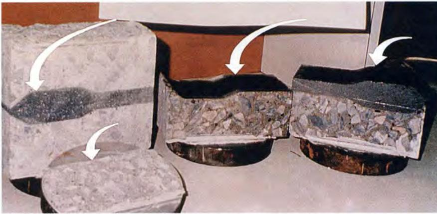
Fig. 10. Comparative failure modes: direct tension composite test.
