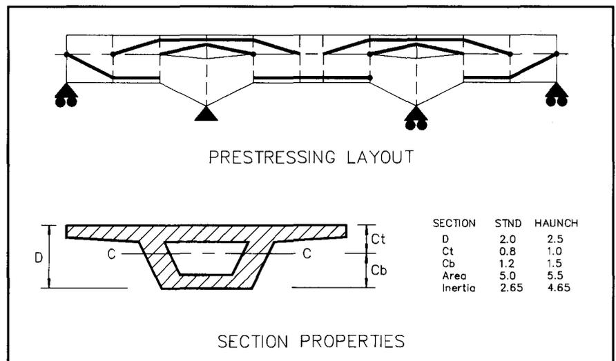
Fig. 9. Three-span bridge example.
