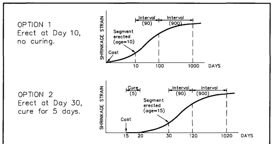
Fig. 2. Relationship of shrinkage to start and curing times.
