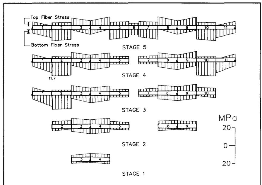
Fig. 12. Top and bottom stresses for various construction stages.
