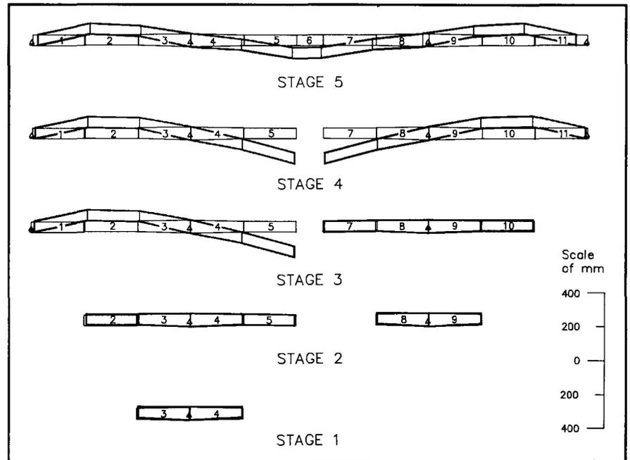
Fig. 11. Deflected shapes for various construction stages.
