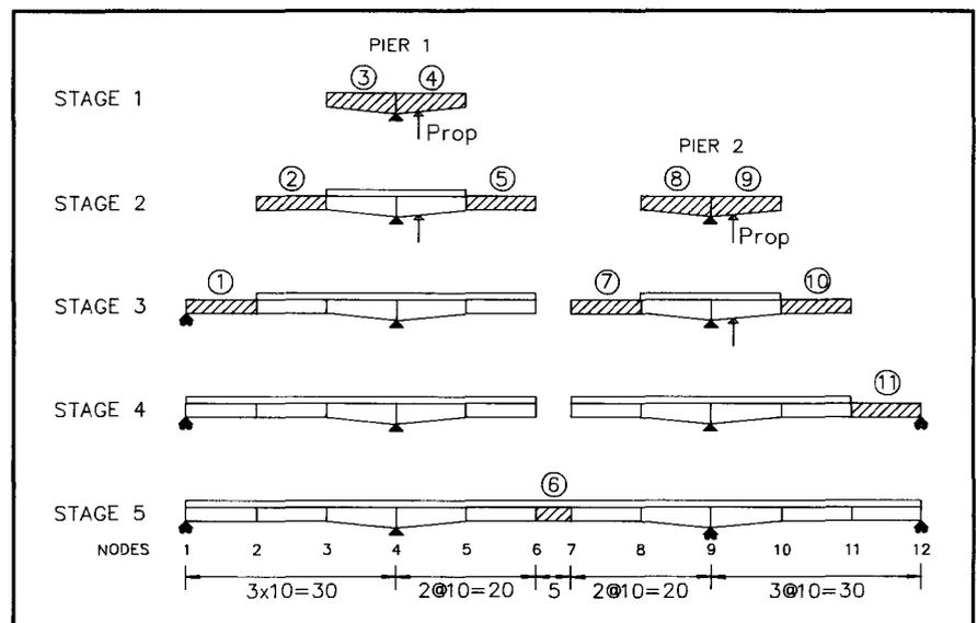
Fig. 10. Construction stages for example bridge.
