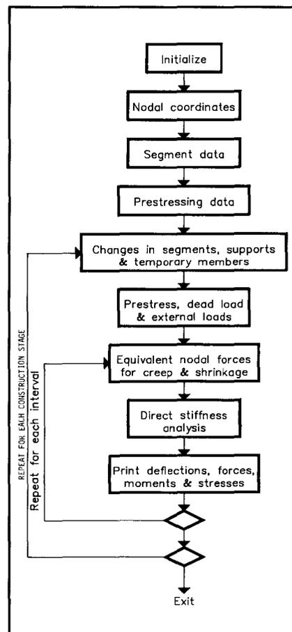
Fig. 7. Simplified program logic diagram.
