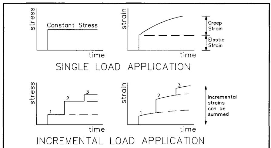
Fig. 1. Superposition of creep effects.
