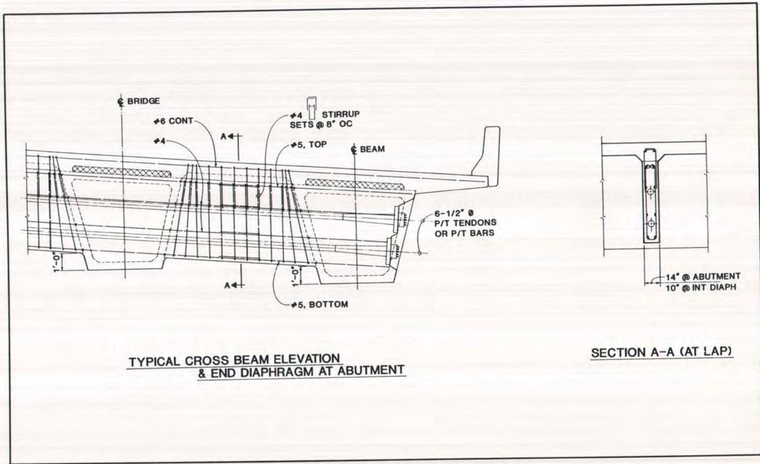
Fig. A4. Precast prestressed concrete horizontally curved bridge beams (cross beam details).
