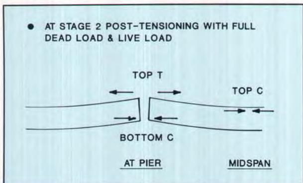
Fig. 12. Critical stress condition (Stage 2).
