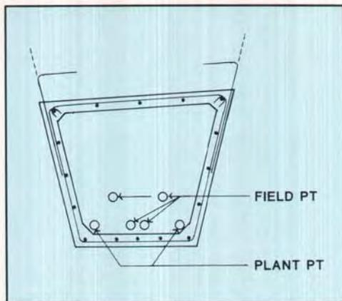
Fig. 15. Reinforcement at typical section.
