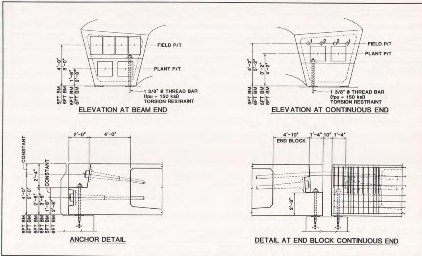
Fig. A7. Precast prestressed concrete horizontally curved bridge beams (sections and details).
