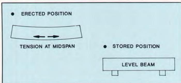
Fig. 10. Critical stress condition (at plant).
