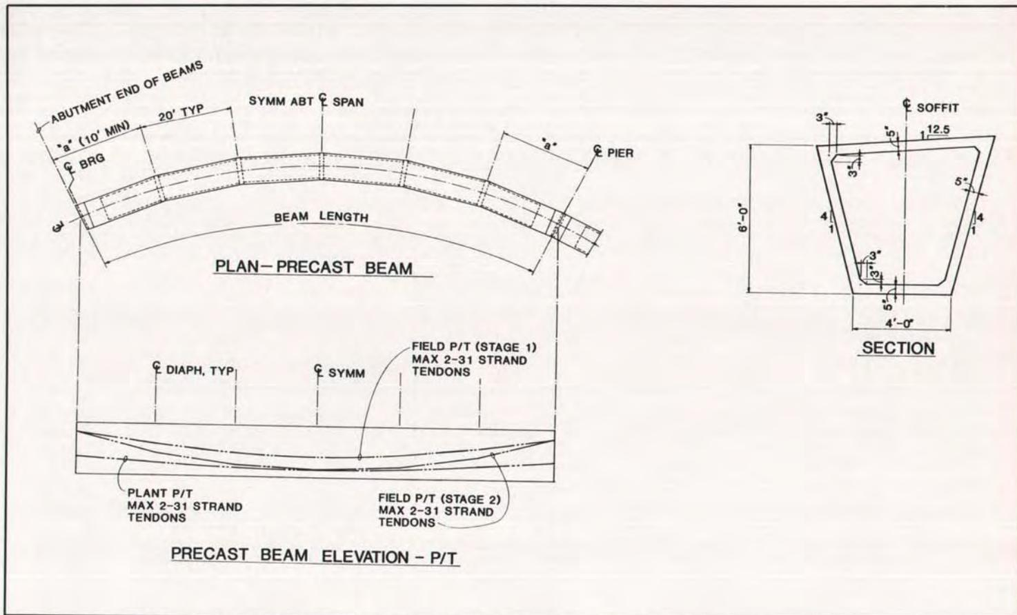
Fig. A3. Precast prestressed concrete horizontally curved bridge beams [6 ft (1.83 m) beam].
