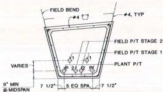
REINFORCEMENT AT TYP SECTION
