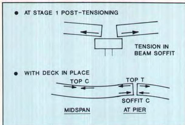
Fig. 11. Critical stress condition (Stage 1).
