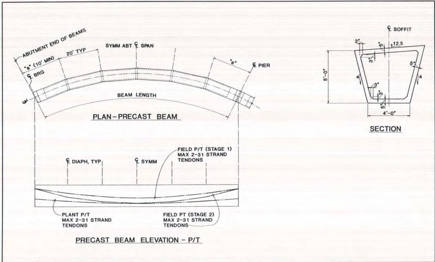
Fig. A2. Precast prestressed concrete horizontally curved bridge beams [5 ft (1.52 m) beam].
