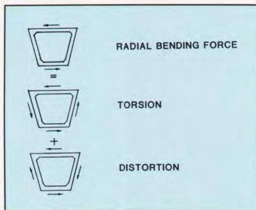
Fig. 14. Torsion/distortion forces.
