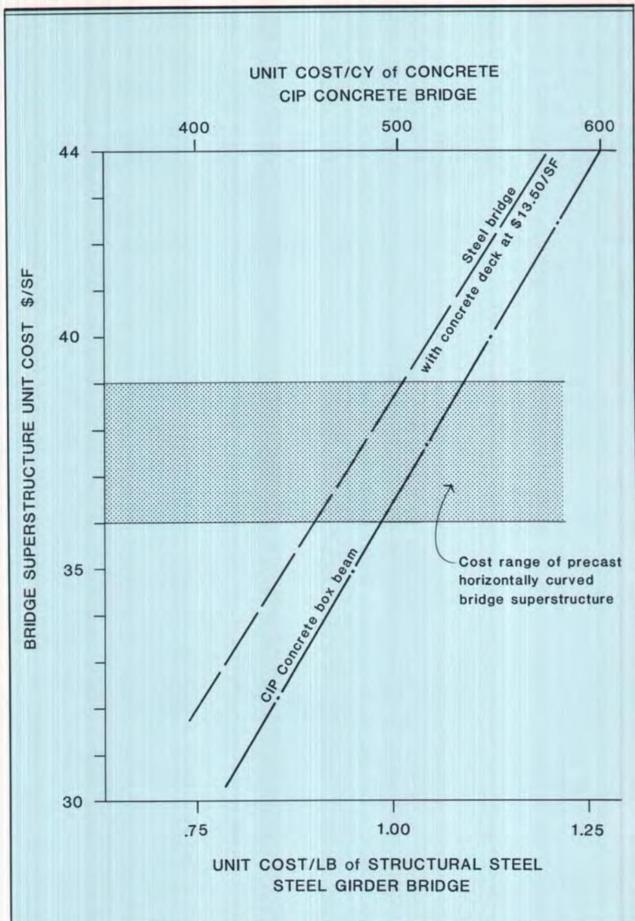
Fig. 8. Comparison of unit superstructure costs. Precast concrete beam bridge versus steel girder bridges and cast-in-place concrete bridges.
