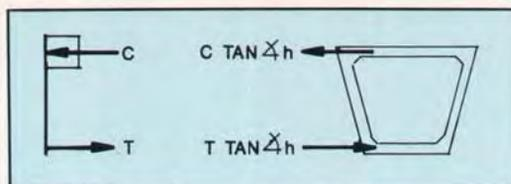
Fig. 13. Radial forces due to turning flexural forces.
