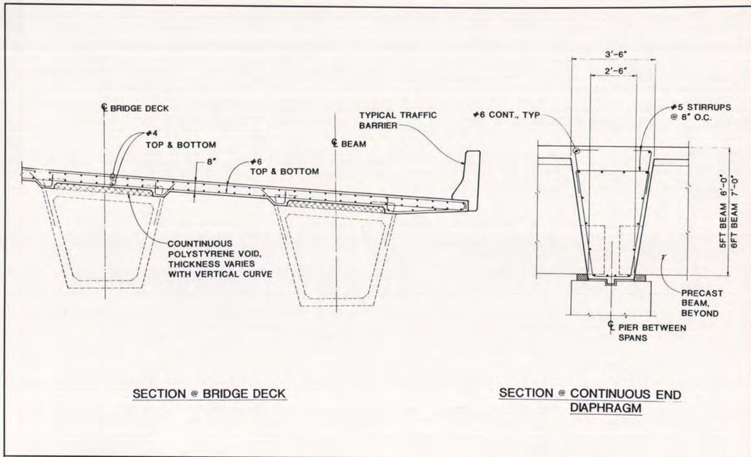
Fig. A5. Precast prestressed concrete horizontally curved bridge beams (deck and pier diaphragm details).
