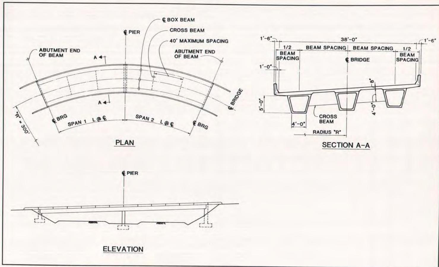
Fig. A1. Precast prestressed concrete horizontally curved bridge beams (typical bridge layout).
