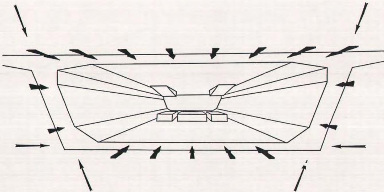
Fig. 12. Basic principles used in strengthening box girders.
