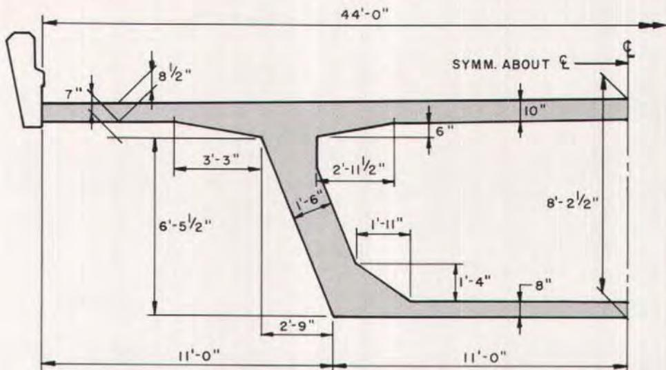
Fig. 3. Cross section of box girder.
