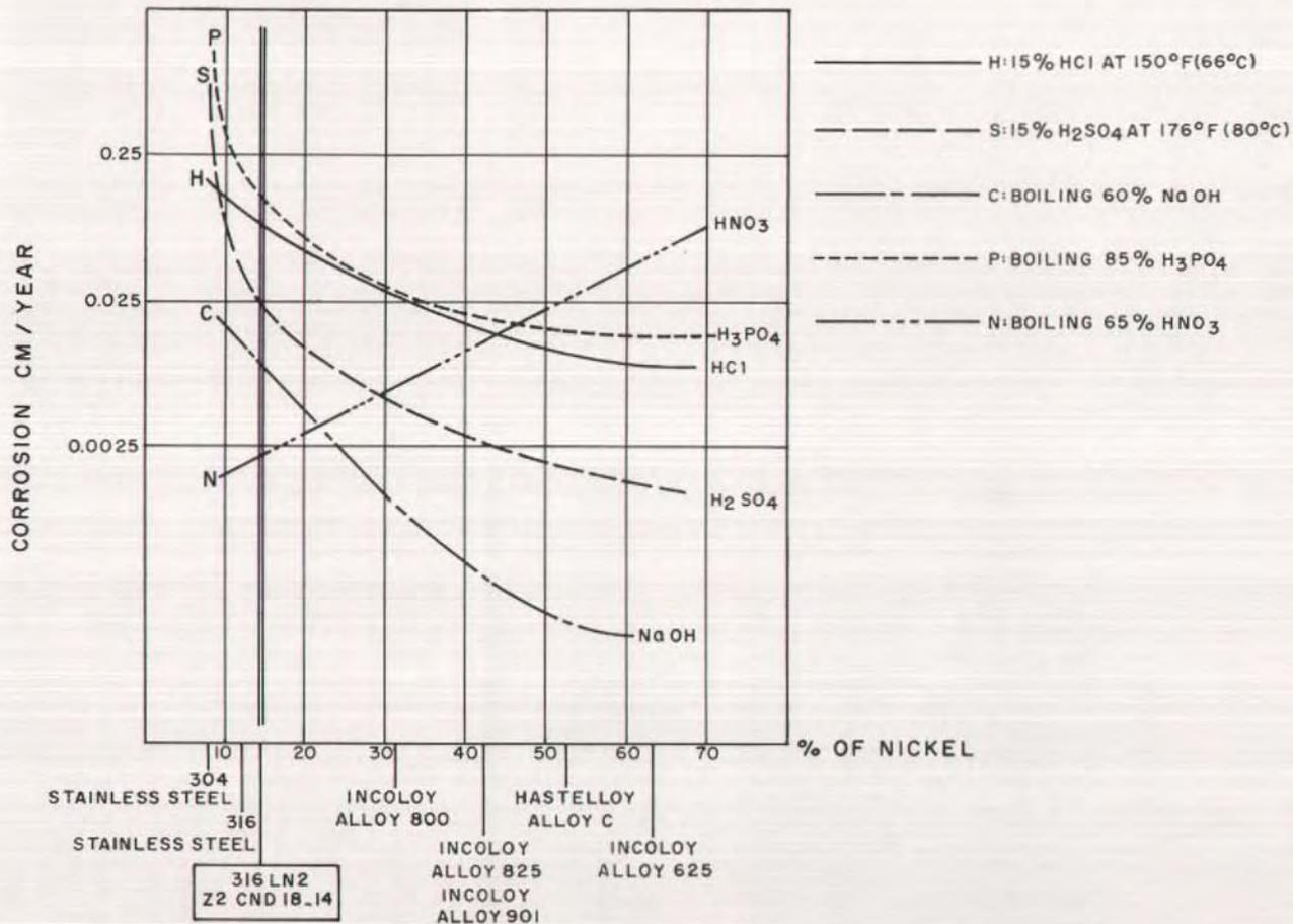
Fig. 16. Corrosion resistance of various steels.
