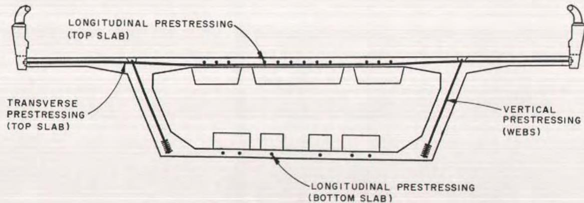
Fig. 5. Tendon locations as provided in original structure.
