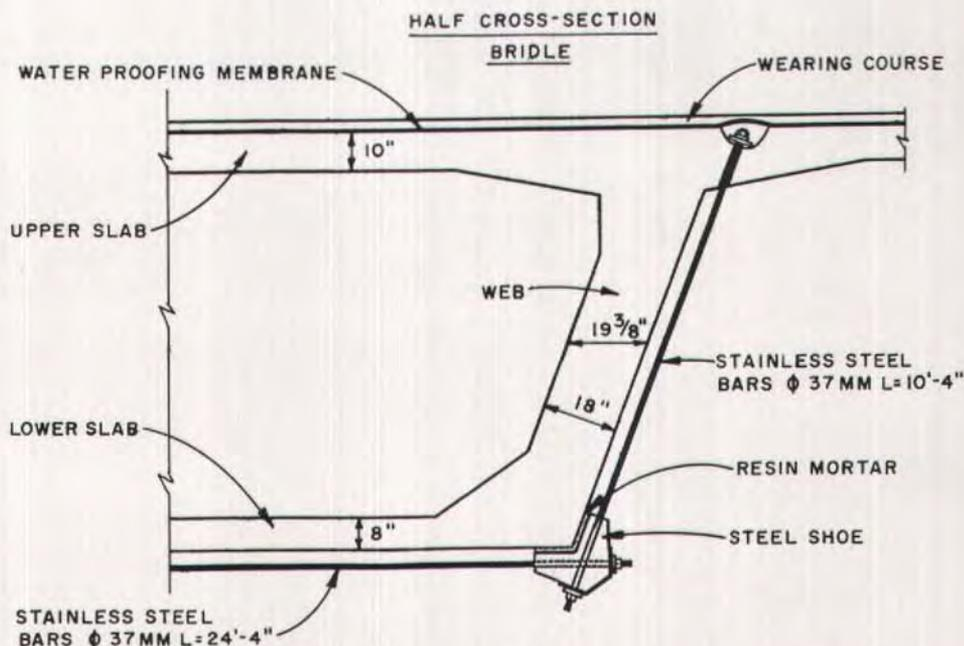
Fig. 13. Vertical and horizontal tendons employed to re-establish integrity of juncture of web and slabs.
