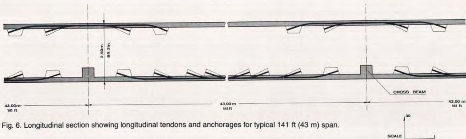
Fig. 6. Longitudinal section showing longitudinal tendons and anchorages for typical 141 ft (43 m) span.
