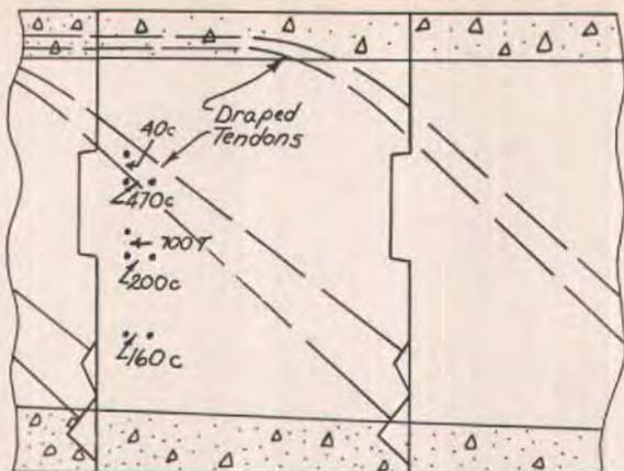
Fig. 23. Strain measurements at a typical alignment key. Note that figures are strains in  $1 \times 10^{-6}$  in./in.
