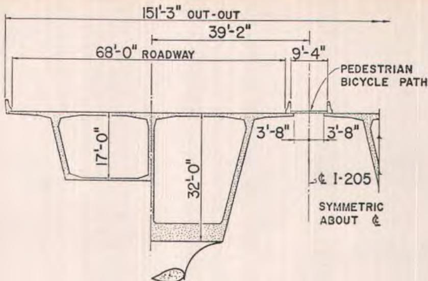
Fig. 7. Cross sections through the value engineering redesign of 600-ft (183 m) main span with the 32-ft (9.76 m) depth at the pier and 17-ft (5.18 m) depth at the midspan.
