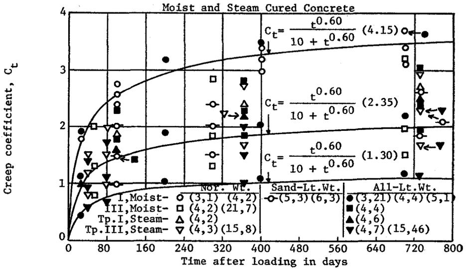
Fig. 2. Creep coefficient vs. time, comparing Eq. (9) with published data. Upper, lower and average values are plotted. All data reduced to "standard" conditions using correction factors. Legend (3, 21) indicates Reference 3 and 21 data points.
