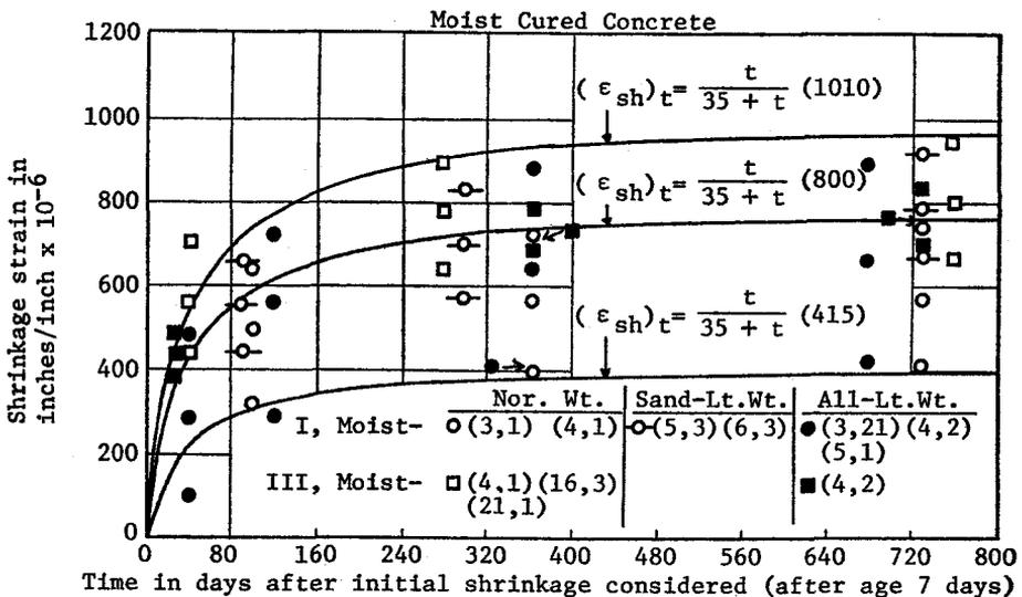
Fig. 3. Shrinkage strain vs. time, comparing Eq. (10) with published data. Upper, lower and average values are plotted. Data reduced to "standard" conditions using correction factors. Legend (3, 21) indicates Reference 3 and 21 data points.
