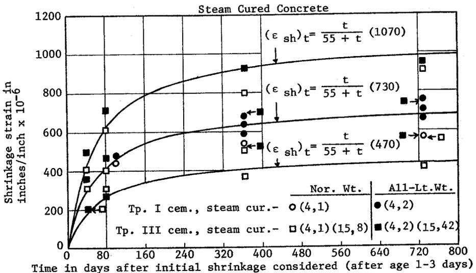
Fig. 4. Shrinkage strain vs. time, comparing Eq. (11) with published data. Upper, lower and average values are plotted. All data reduced to "standard" conditions using correction factors. Legend (15, 8) indicates Reference 15 and 8 data points.
