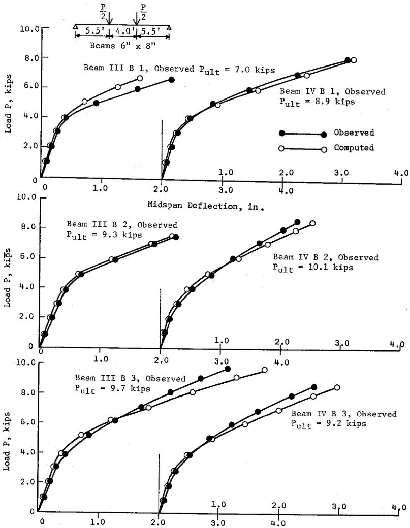
Fig. 11. Experimental and computed loss vs. mid-span deflection for the Series III and IV beams of Reference 34
