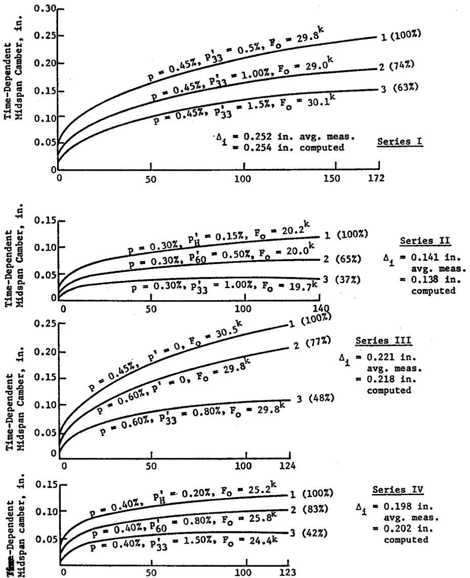
Fig. 9. Experimental time-dependent mid-span camber for 12 test beams
