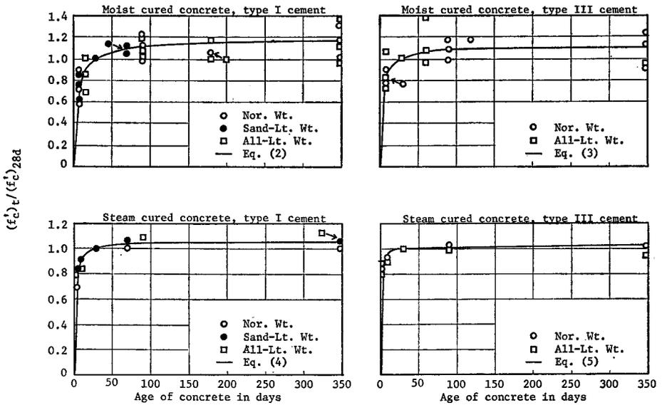
Fig. 1. Concrete strength vs. time, comparing Eqs. (2) to (5) with experimental data from References 1 to 6. Where three data points are shown for a given age, they refer to upper, lower and average values for a given set of data. Where only one data point is shown, the range is too small to indicate. Data for 88 specimens are included.
