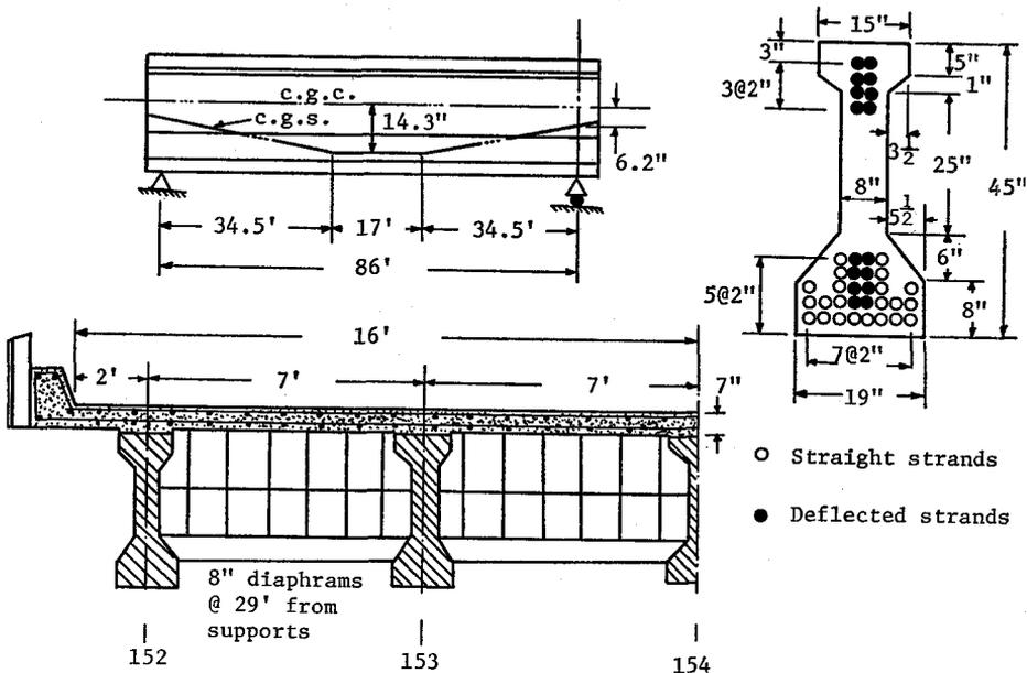
Fig. 5. Sand-lightweight concrete prestressed bridge girders composite with normal weight concrete deck slab
