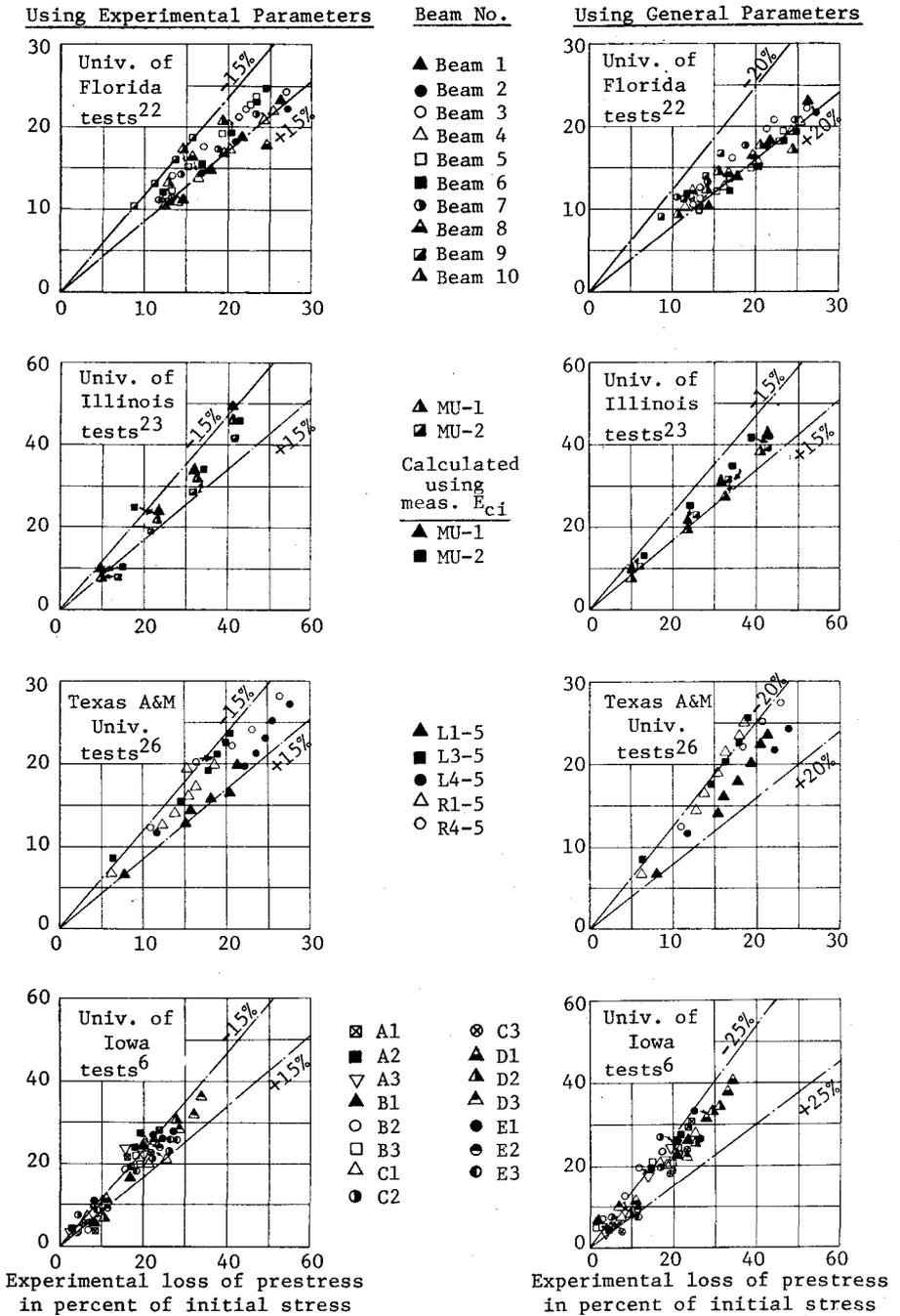
Fig. 7. Comparison of experimental and computed mid-span loss of prestress at various ages.
