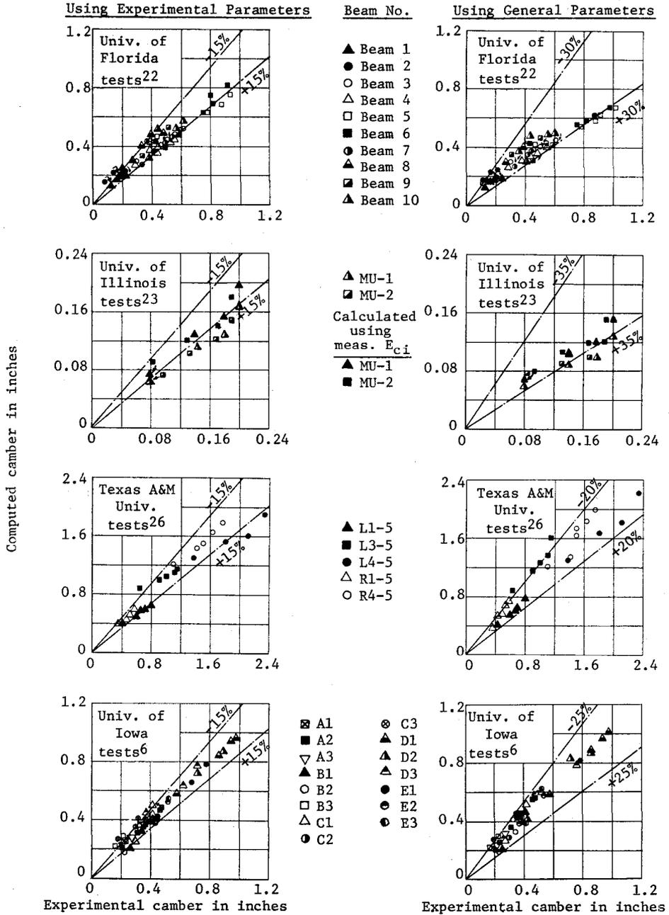
Fig. 8. Comparison of experimental and computed mid-span camber at various ages.
