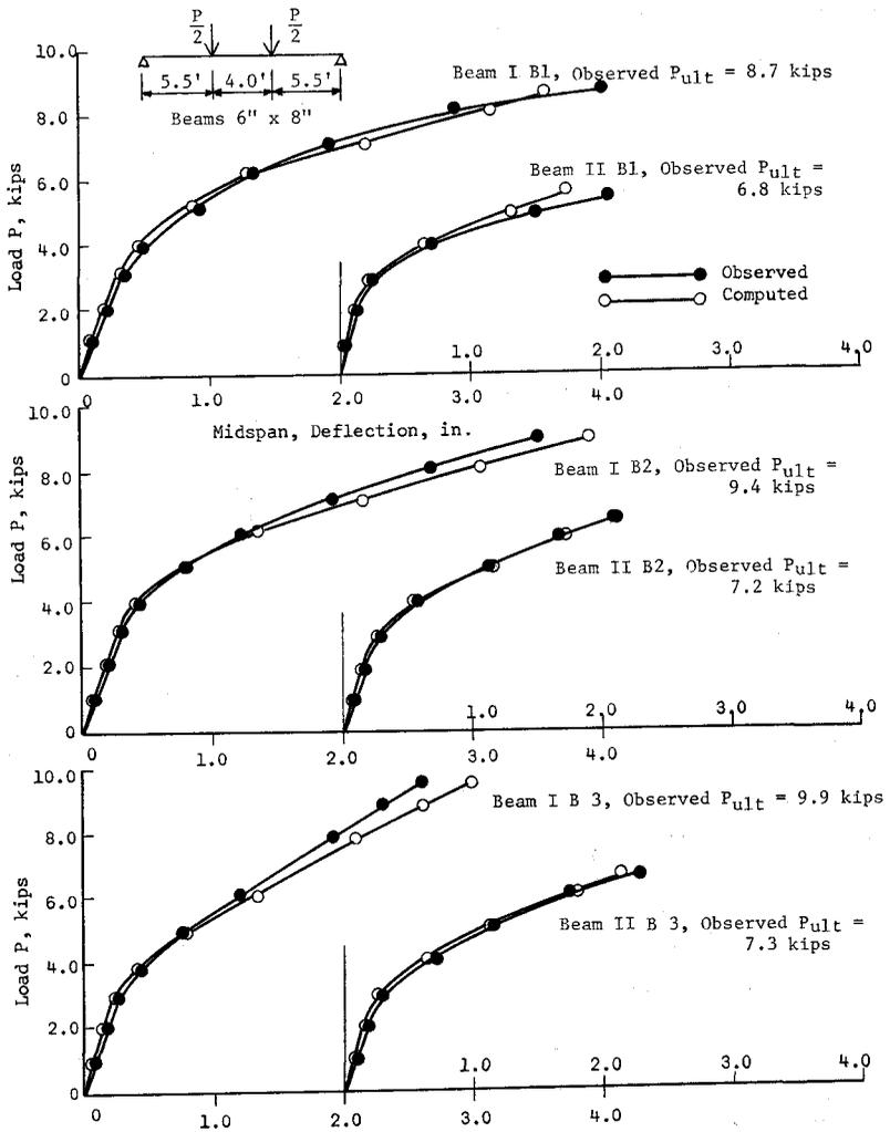
Fig. 10. Experimental and computed loss vs. mid-span deflection for the Series I and II beams of Reference 34
