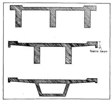
The impression of slenderness can be emphasized by increasing the cantilevered width of the deck slab and by good proportion between the depth of the fascia beam and the depth of the main girder. Fascia beam depth should also be in good proportion with the length of the main span—at least 1/100 of the span length for spans up to 150 ft. or 1/4 to 1/5 of the total depth for longer spans.
