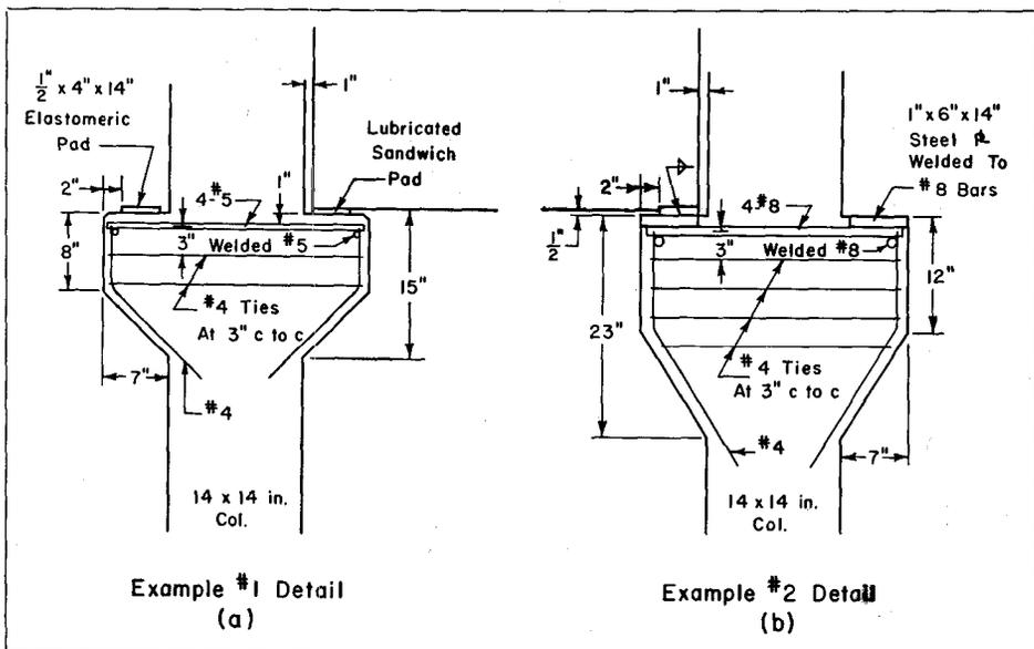
Fig. 4—Corbel Details for Example Problems
