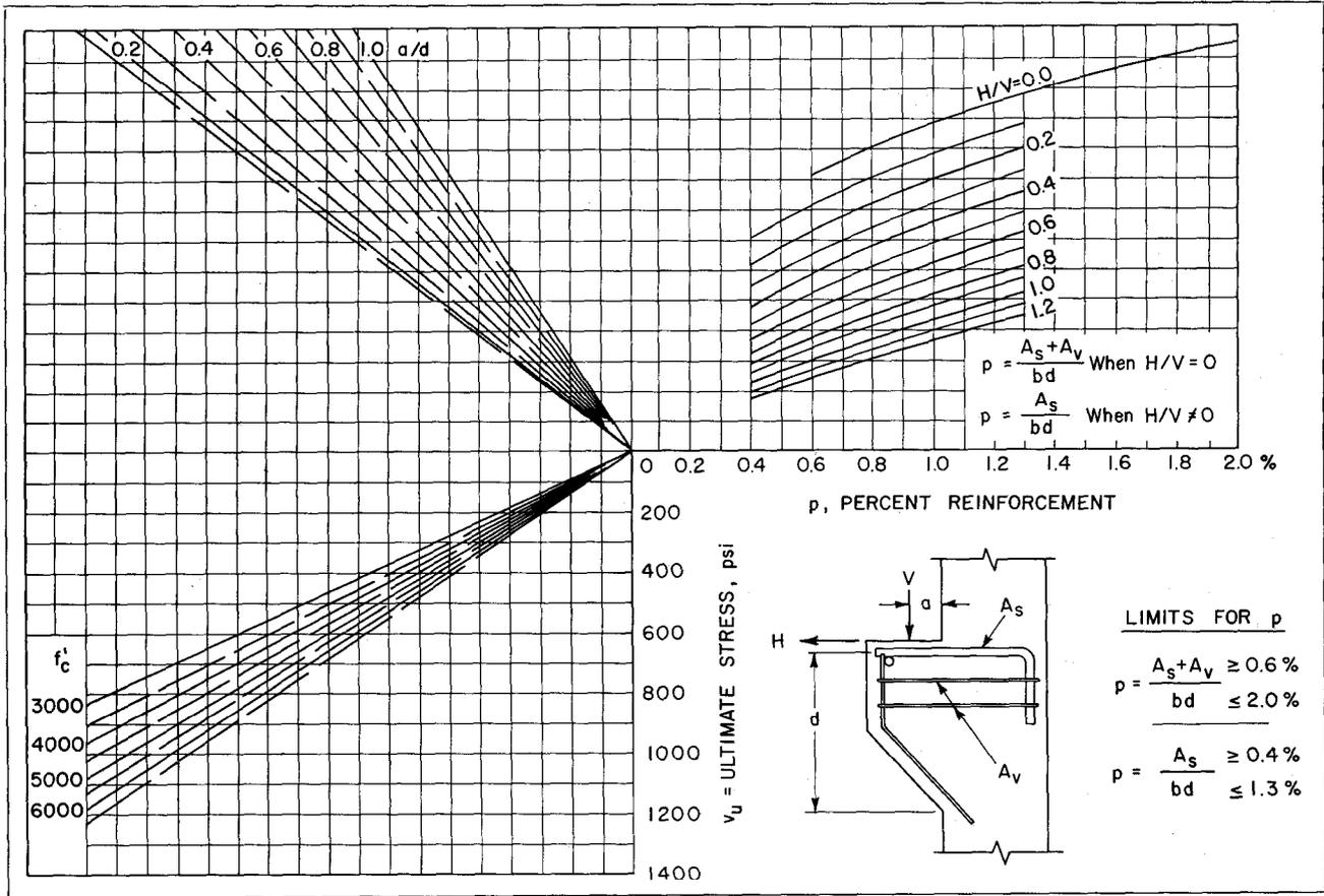
Fig. 3—Design Chart for Ultimate Strength of Corbels
