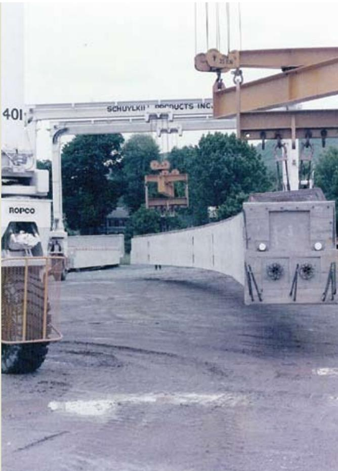
**Figure 2.** The Pennsylvania Department of Transportation used curved, precast, post-tensioned concrete box girders produced by Schuylkill Co. for the Philadelphia Airport renovation. Courtesy of Joseph Nagle, Schuylkill Co.
