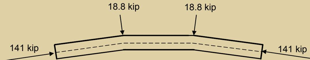
**Figure 15.** After the prestressing strands and the threaded rods were flame cut, the beam was subjected to the self-balanced forces. Note: 1 kip = 4.448 kN.
