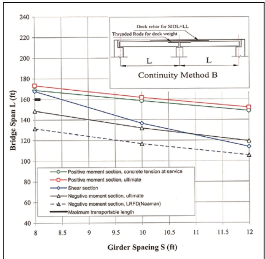
Fig. 1. NU1100 span capacities, System B.
