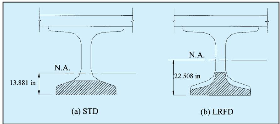
Fig. 3. Compression block area for the example in Fig. 2 according to AASHTO Standard (STD) and LRFD Specifications.
