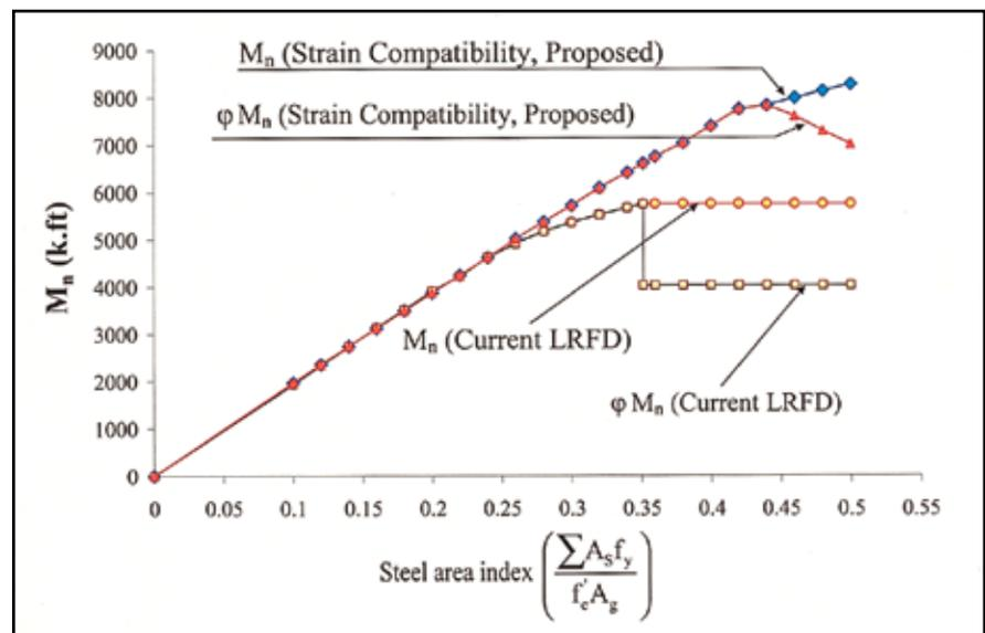
Fig. 4. Proposed strain compatibility design moment for section in Answer A4, versus current AASHTO-LRFD solution.
