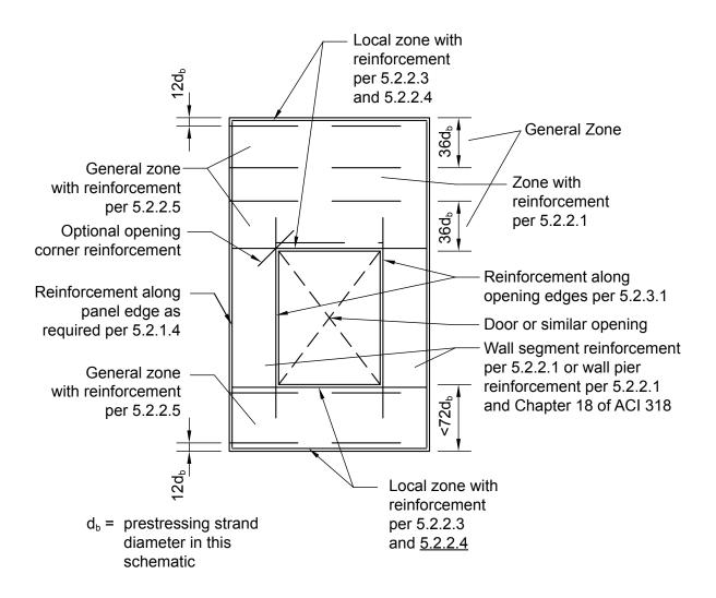
**Page C-7,** Figure C5.2.2.2: Replace "Local zone with reinforcement per 5.2.2.3 and 5.2.2.3" with "Local zone with reinforcement per 5.2.2.3 and 5.2.2.4" at the bottom of the figure.
