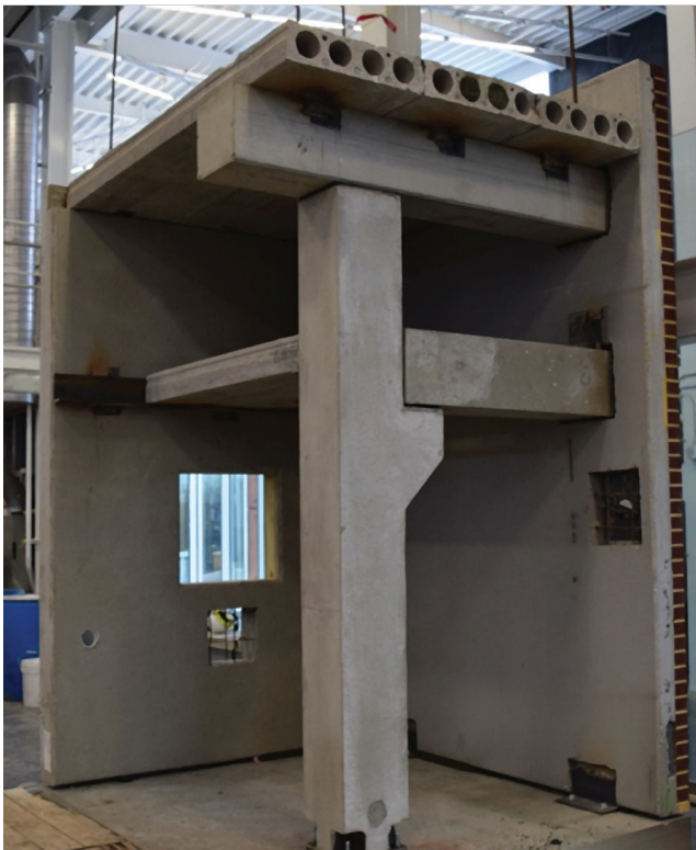
Molin Concrete Products of Lino Lakes, Minn., and the University of Minnesota Duluth designed this precast concrete demonstration structure as a teaching tool, shown from the back, which allows students to observe, touch, and visualize concepts in real time. Courtesy of Ben Dymond.
